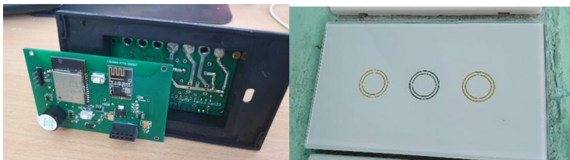
Figure 6. Control panel circuit board inside and buttons outside
