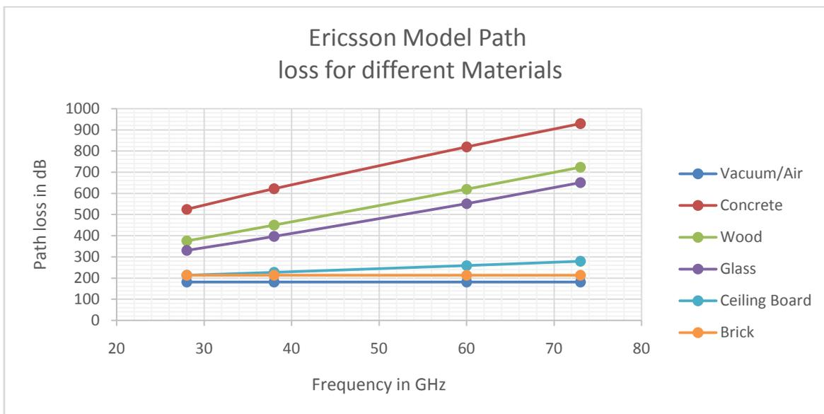
Fig 3: Plot of Pathloss(dB) at 28GHz, 38GHz, 60GHz, 73GHz for Ericsson
