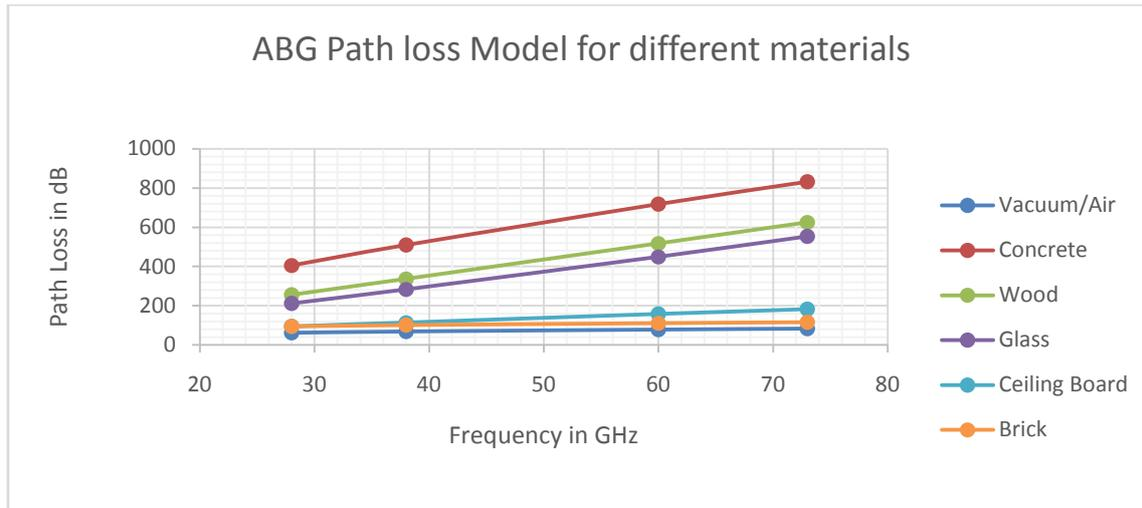
Fig 5: Plot of Pathloss(dB) at 28GHz, 38GHz, 60GHz, 73GHz for ABG
