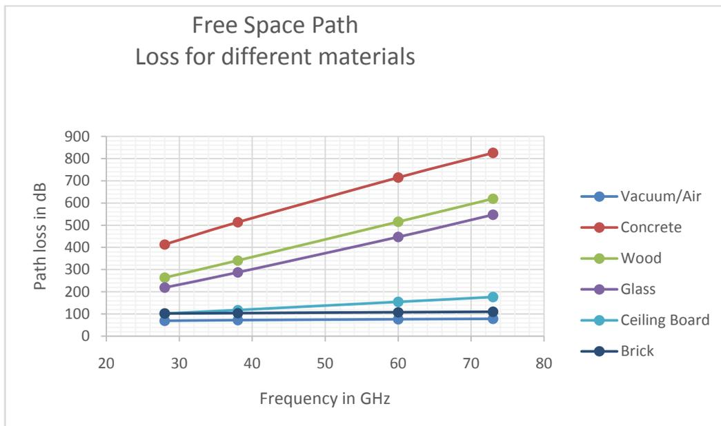
**Fig 1: Plot of Pathloss(dB) at 28GHz, 38GHz, 60GHz, 73GHz for FS**
