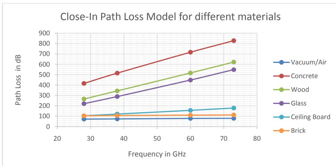
Fig 4: Plot of Pathloss(dB) at 28GHz, 38GHz, 60GHz, 73GHz for CI
