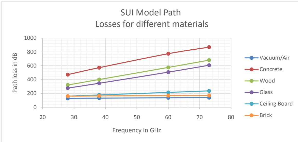
Fig 2: Plot of Pathloss(dB) at 28GHz, 38GHz, 60GHz, 73GHz for SUI
