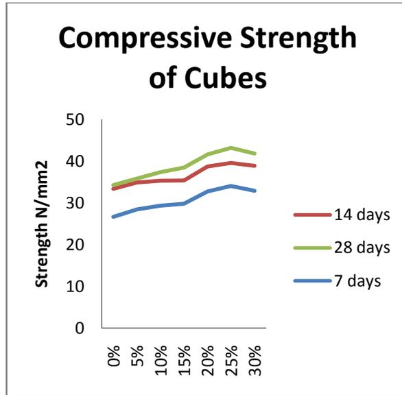
**Fig No.4.1 Impact of Granite Powder on Compressive Strength of Matrix**
