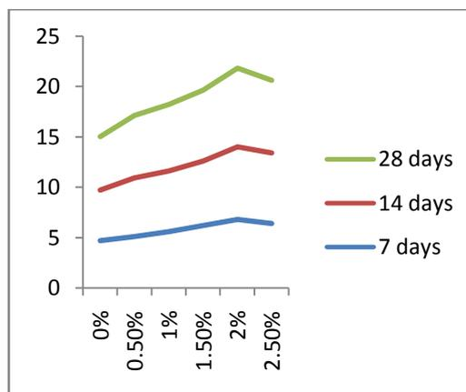
**Fig No.4.6 Impact of Steel Fibers on Flexural strength of Matrix**
