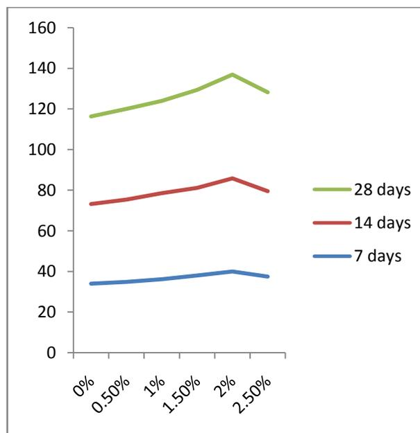
**Fig No.4.2 Impact of Steel Fibers on Compressive Strength of Matrix**
