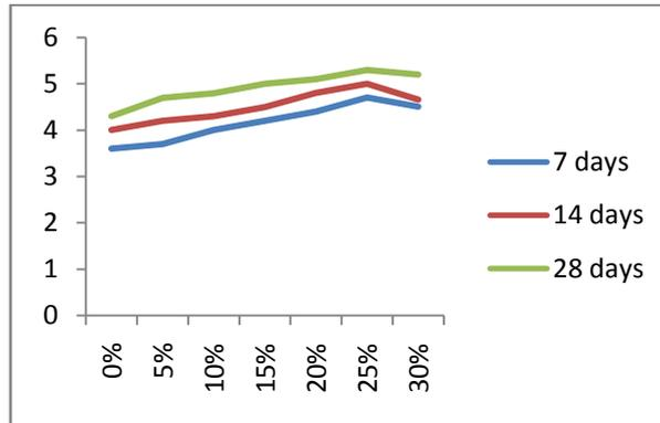
**Fig No.4.5 Impact of Granite Powder on Flexural strength of Matrix**
