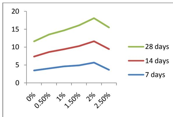
Fig No.4.4 Impact of Steel Fibers on Split Tensile Strength of Matrix
