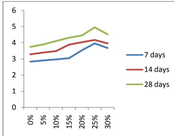
Fig No.4.3 Impact of Granite Powder on Split Tensile Strength of Matrix
