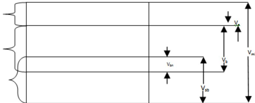
Figure 1 Density – Voids relationships of a compacted specimen of asphalt paving mix.
