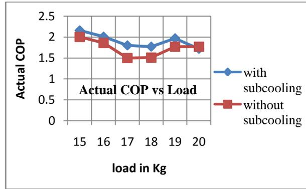
From the graph it is observed that when load on the evaporator is varied there is increase in actual COP when TEC is integrated with VCR system for subcooling of refrigerant. For 18Kg load on evaporator there is maximum increase in actual COP is 17.21854%.
