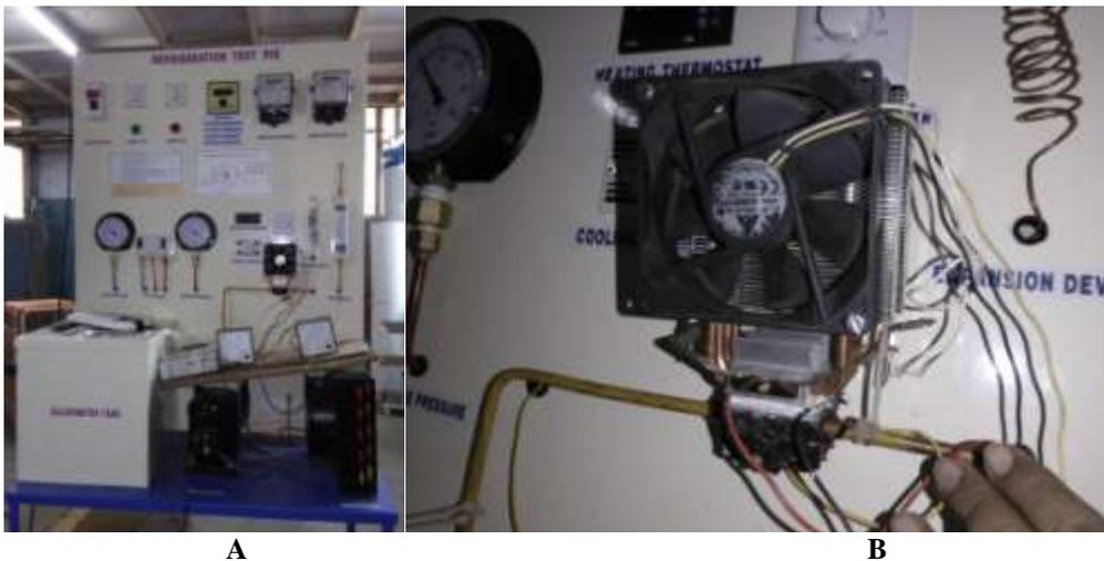
**Fig No 1 A. Experimental Setup, B TEC Module with Heat Pipe**
