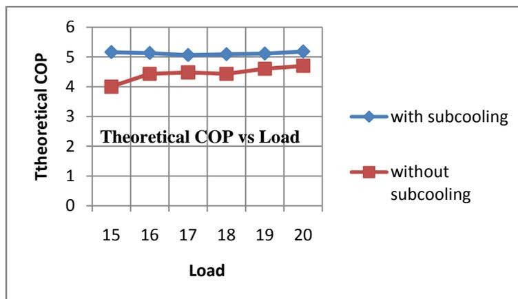
From the graph it is observed that when load on the evaporator is varied there is increase in theoretical COP when TEC is integrated with VCR system for subcooling of refrigerant. For 15Kg load on evaporator there is maximum increase in actual COP 15.95%.
