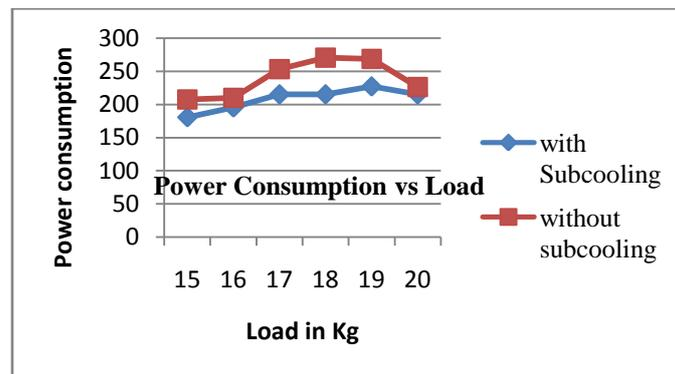
From the graph it is observed that when load on the evaporator is varied there is reduction in power consumed when TEC is integrated with VCR system for subcooling of refrigerant. for 18Kg load on evaporator there is maximum reduction in power consumption is 20.40%.
