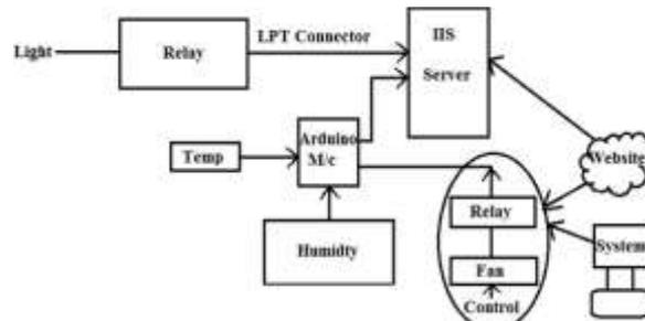
**figure 2** block diagram of smart building architecture
