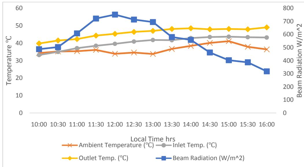
Figure 5 Temperature Variation with Beam Radiation of Double-Glazed Flat plate
