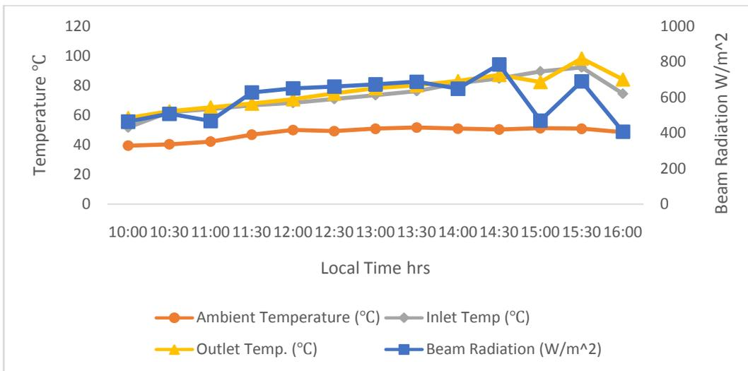
Figure 2 Temperature Variation with Beam Radiation for Evacuated Tube at 30<sup>0</sup>
