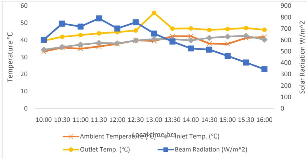
Figure 4 Temperature Variation with Beam Radiation for Triple-glazed Flat Plate
