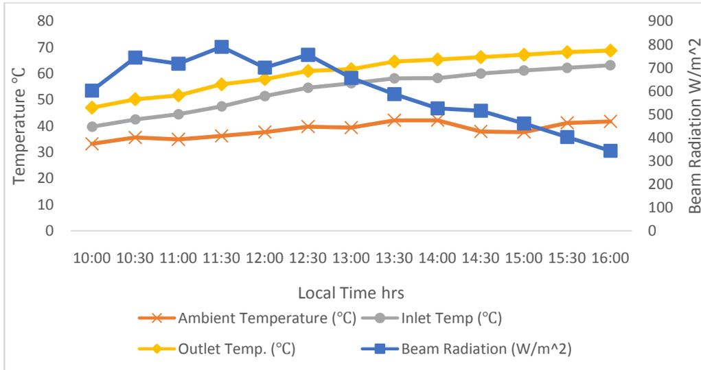
Figure 1 Temperature Variation with Beam Radiation for Evacuated Tube at 45<sup>0</sup>
