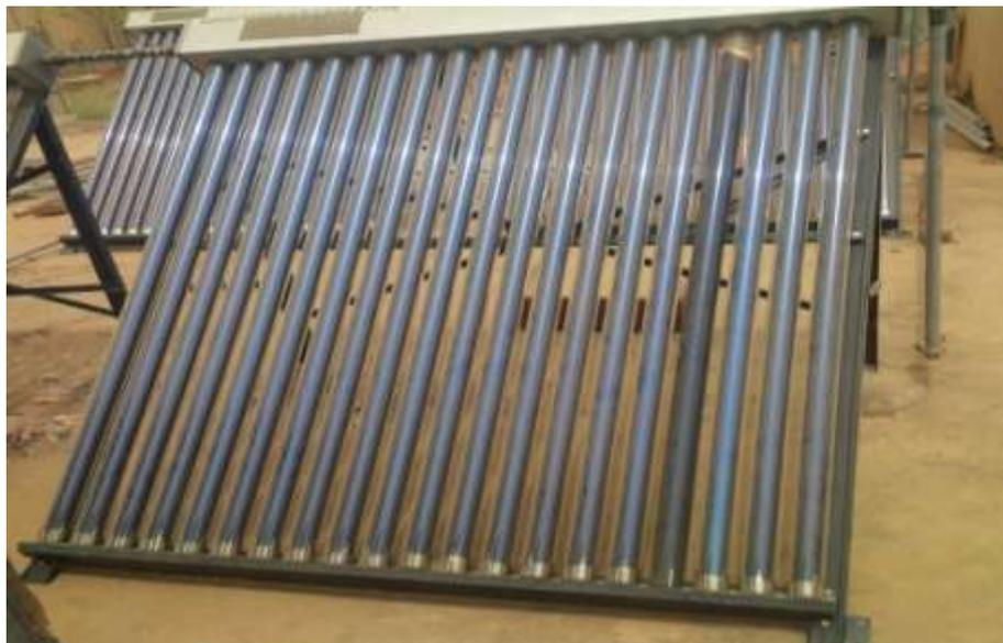
**Figure 3** Evacuated Tube Solar Water Heater tilted at 45° at Sokoto Energy Research Centre.
