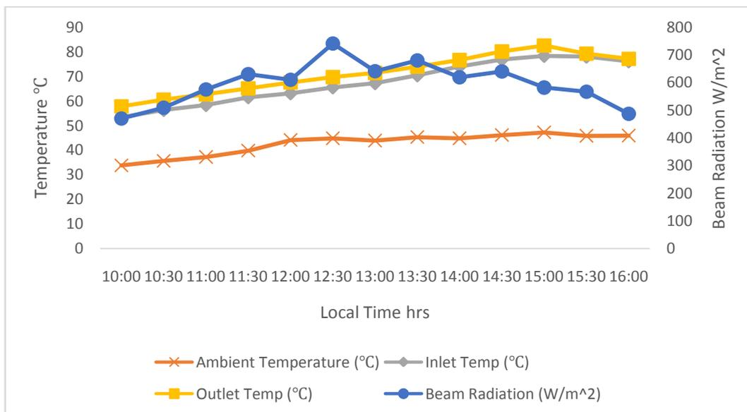
Figure 3 Temperature Variation with Beam Radiation for Evacuated Tube at 15<sup>0</sup>
