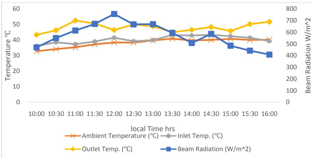
Figure 6 Temperature Variation with Beam Radiation for Single-glazed Flat Plate
