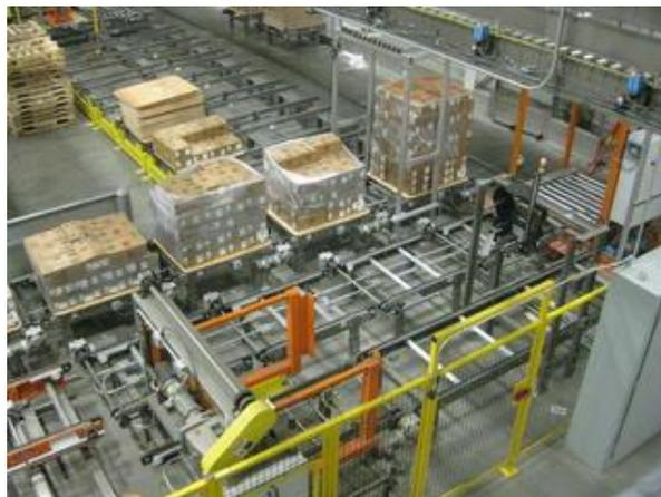
**Figure II Pallet Handling Conveyor Systems.**
