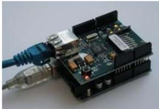
Fig.5 Arduino Duemilanove and Ethernet Shield
