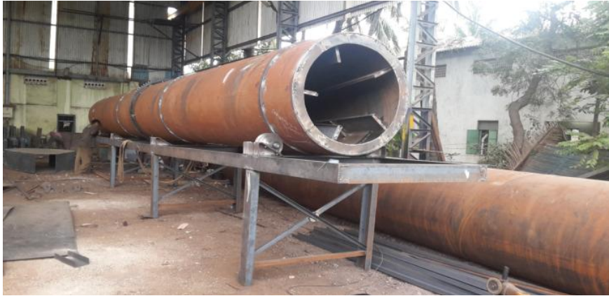
Fig.1 Rotary Drum with Five Flights used for Drying Bagasse.
