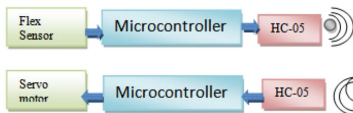
Figure 1: Block Diagram of the prototype
