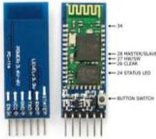
HC-05 module is an easy to use Bluetooth SPP (Serial Port Protocol) module, designed for transparent wireless serial connection setup. Serial port Bluetooth module is fully qualified Bluetooth V2.0+EDR (Enhanced Data Rate) 3Mbps Modulation with complete 2.4GHz radio transceiver and baseband. It uses CSR Bluecore 04-External single chip Bluetooth system with CMOS technology and with AFH (Adaptive Frequency Hopping Feature). It has the footprint as small as 12.7mmx27mm
