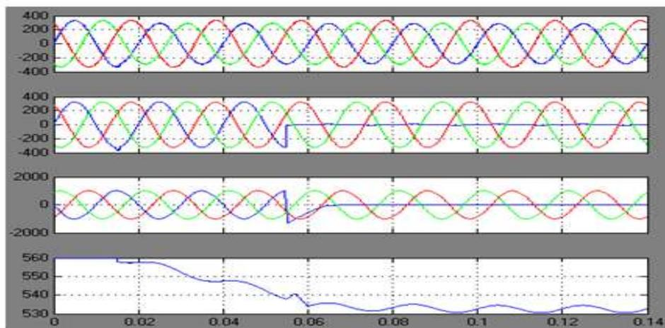
**Fig.17.**(a) Source voltages. (b) Load voltages. (c) Line currents. (d) DC-link voltage, during phase-A to ground downstream fault which takes place during sag compensation in phases A and B.
