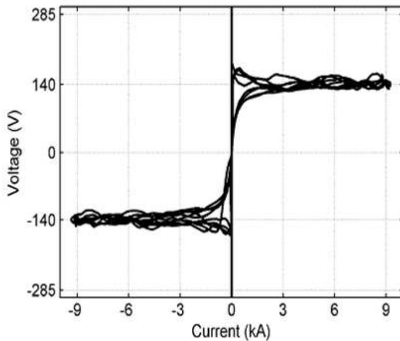
**Fig. 14.** Nonlinear v-i characteristic of the arc.
