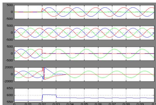
**Fig.10.(a)** Injected voltages. (b) Source voltages. (c) Load voltages. (d) Line currents. (e) DC-link voltage, during the phase-to-phase downstream fault.
