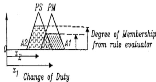
**Fig.4.** Defuzzification using center of gravity method.
