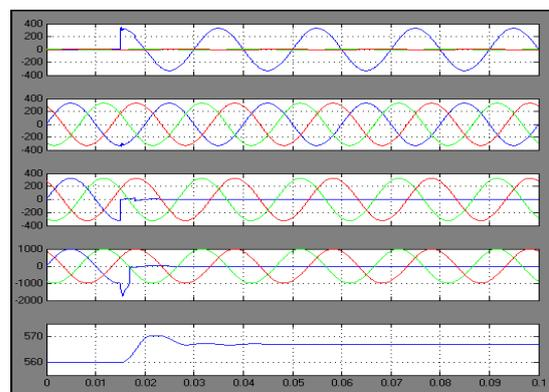
**Fig.16.**(a)Injected voltages.(b)Source voltages.(c) Load voltages. (d) Line currents. (e) DC-link voltage, during the single-phase-to-ground downstream arcing fault.
