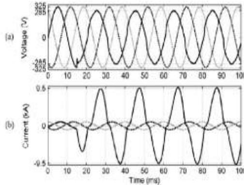
**Fig.13.** (a) Voltages at Bus3 (b) Fault currents, during the downstream single phase-to-ground arcing fault when the DVR is inactive (bypassed).
