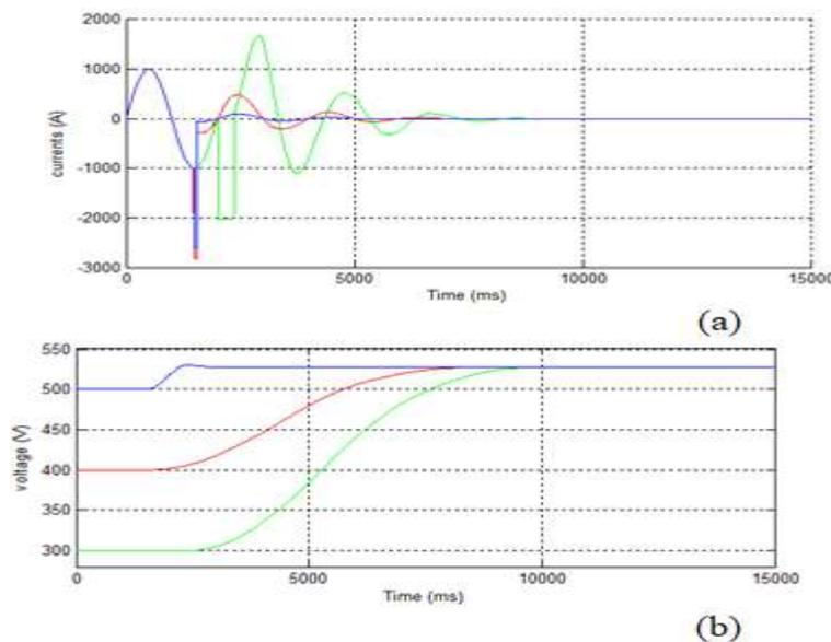
**Fig.18.**(a) Line current of phase-A and (b) dc-link voltage, for different initial values of the dc-link voltage, during downstream phase-A-to-ground fault.
