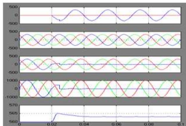
**Fig.12.**(a) Injected voltages. (b) Source voltages. (c) Load voltages. (d) Line currents. (e) DC-link voltage, during the single-phase-to-ground downstream fault.
