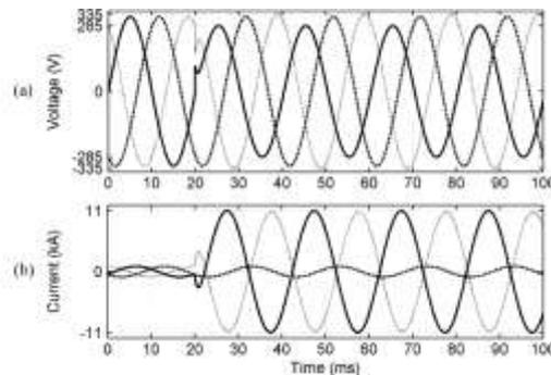
**Fig.9.(a)** Voltages at bus 3, (b) Fault currents, during downstream phase-to-phase downstream fault when the DVR is inactive (bypassed).
