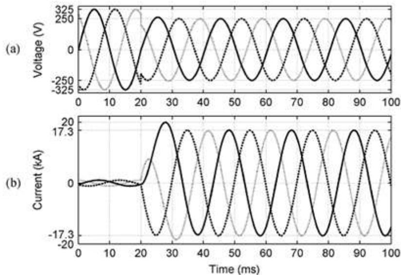
Fig.7.(a) Voltages at bus3 (b) Fault currents, during downstream three-phase fault when the DVR is inactive(bypassed).
