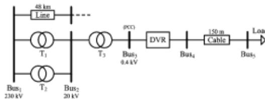
Fig.6. Single-line diagram of the system used for simulation studies
