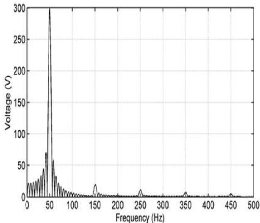
**Fig.15.** Harmonic content of voltage at during the arcing fault
