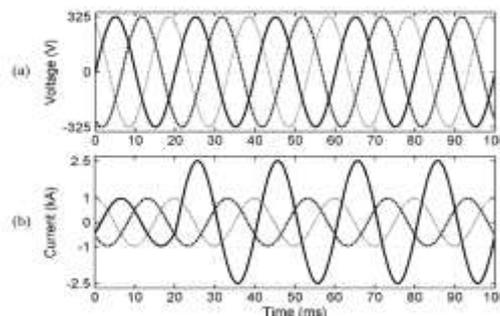
**Fig.11.** (a) Voltages at Bus3 (b) Fault currents, during the downstream single phase-to-ground fault when the DVR is inactive (bypassed).
