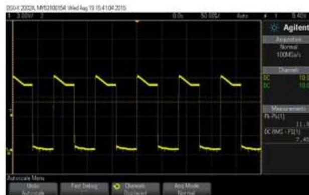
Figure 14: Pulses to  $S_a$
