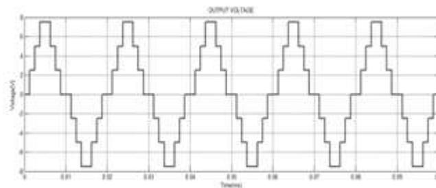
Figure 6: Output voltage (Asymmetric)
