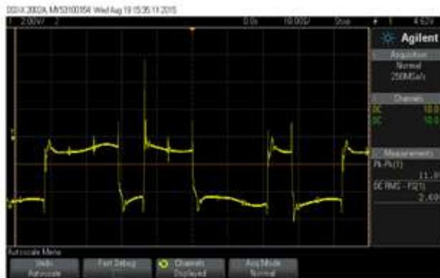
Figure 15: Voltage stress across  $S_{L11}$
