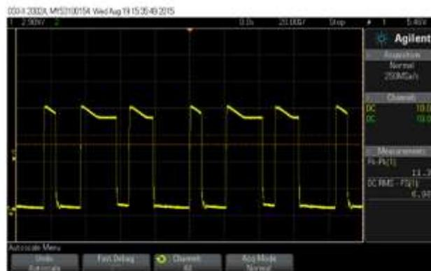
Figure 13: Pulses to  $S_{R11}$
