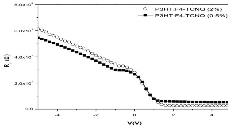
**Figure 5.**The frequency dependent  $R_i$ -V characteristic comparison of 0.5% and 2% F4-TCNQ concentration used Au/P3HT:F4-TCNQ/n-Si SBDs at 1MHz.
