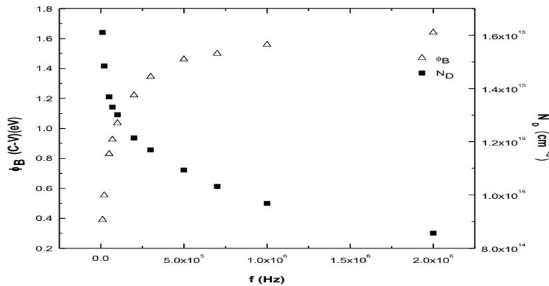
**Figure 11.** The  $\phi_B$  (C-V) and  $N_D$  parameters for various frequencies for the Au/P3HT:F4-TCNQ/n-Si Schottky barrier diode
