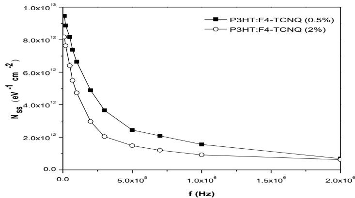
**Figure 6.** The frequency dependent  $N_{ss}$  characteristic for 2% and 0.5% F4-TCNQ concentration used Au/P3HT:F4-TCNQ/n-Si MPS SBDs.
