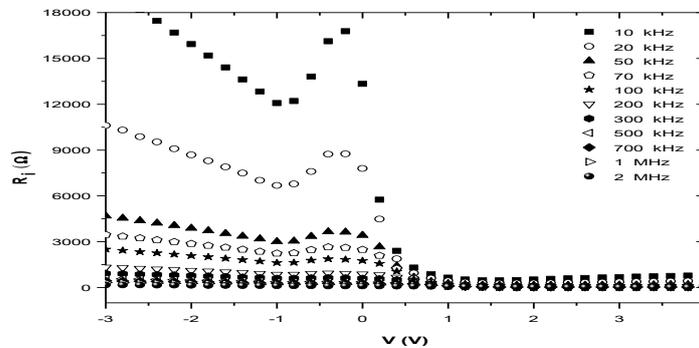
**Figure 9.**The characteristics of diode resistance ( $R_i$ ) for various frequencies of the Au/P3HT:F4-TCNQ/n-Si Schottky barrier diode at room temperature.
