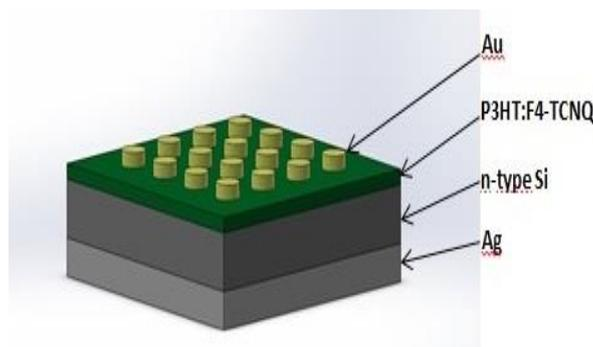
**Figure 1.** Au/P3HT:F4-TCNQ/n-Si diode structure.
