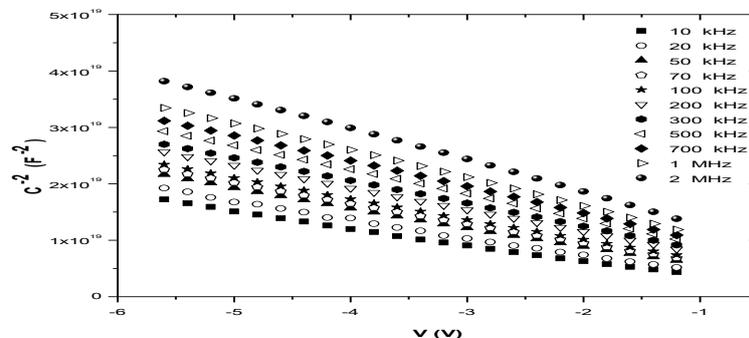
**Figure 10.**The  $C^{-2}$ -V plots of the Au/P3HT:F4-TCNQ/n-Si Schottky barrier diode at room temperature as a function of voltage
