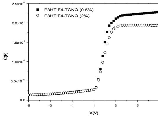
**Figure 4.**The F4-TCNQ concentration dependent capacitance-voltage characteristic for Au/P3HT:F4-TCNQ/n-Si MPS SBDs at 1MHz.
