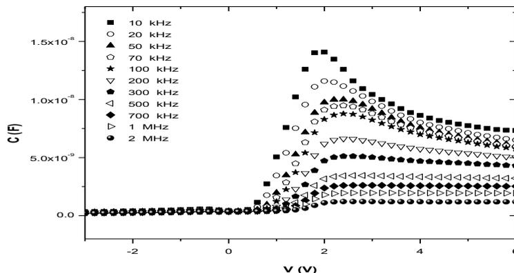
**Figure 7.** The frequency dependent capacitance-voltage characteristic of 2% F4-TCNQ used Au/P3HT:F4-TCNQ/n-Si SBD.
