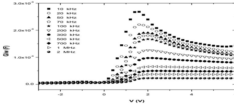
**Figure 8.**The frequency dependent conductance-voltage characteristic of 2% F4-TCNQ used Au/P3HT:F4-TCNQ/n-Si SBD.
