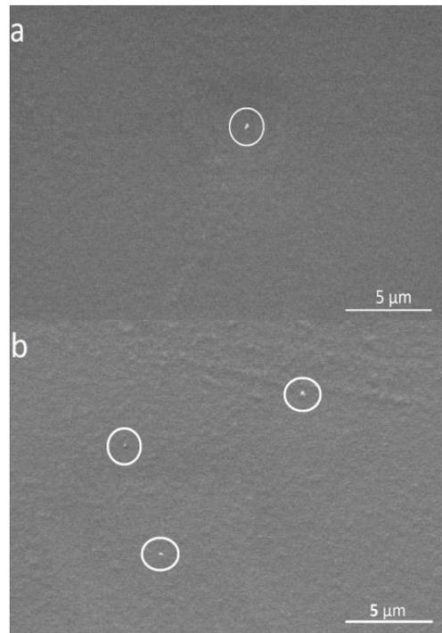
Figure 2. SEM images of (a) 0.5% F4-TCNQ and (b) 2% F4-TCNQ concentration used P3HT:F4-TCNQ surfaces.
