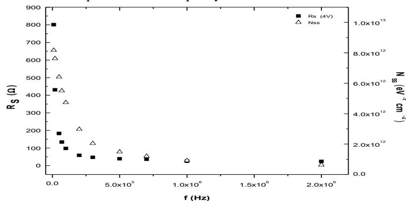
**Figure 12.** The variation of  $N_{ss}$  and  $R_s$  for various frequencies for the Au/P3HT:F4-TCNQ/n-Si Schottky barrier diode
