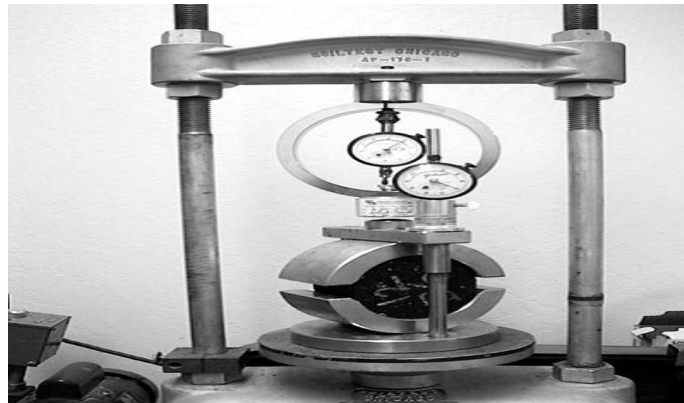
Figure 3.1 Marshall Test Setup
