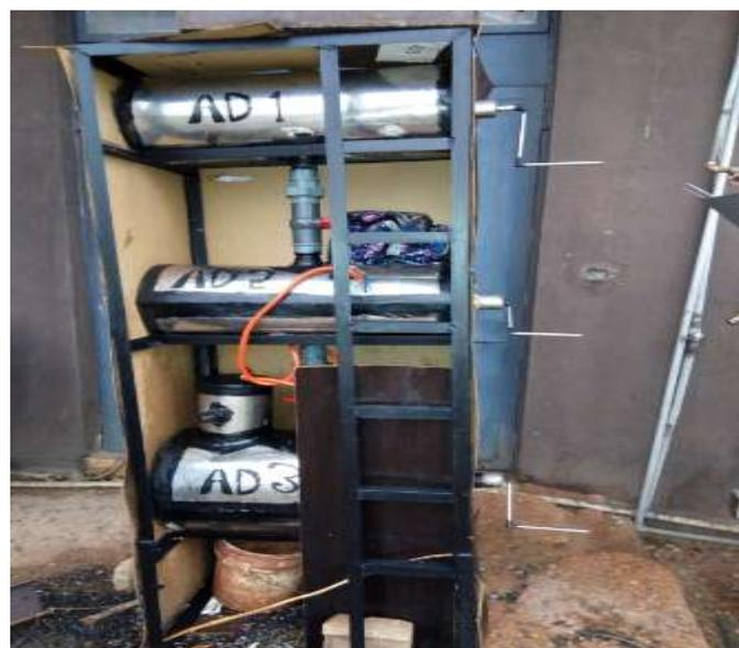
**Figure 3** Three Stages Continuous AD Plant
