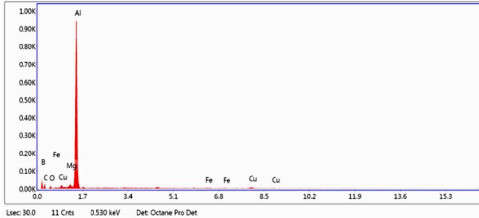
Figure 3b: EDS spectrum of Al-2024 alloy and 4%  $B_4C$
