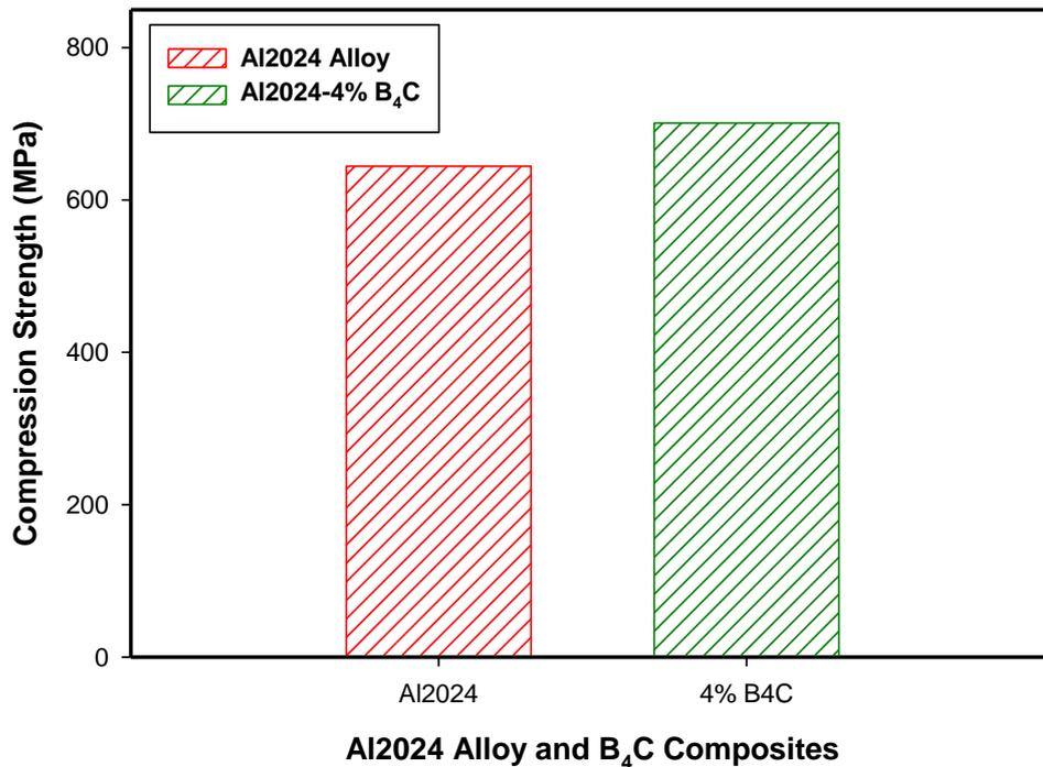
**Figure 5:** Compression strength of Al2024 and 4 wt. % of micro B<sub>4</sub>C composites
