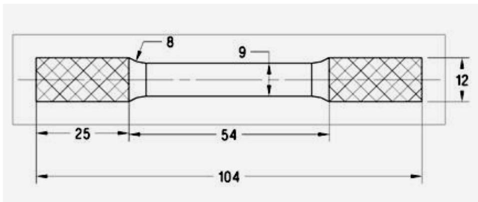
**Figure 1:** Tensile specimen according to ASTM E8 with all dimensions in mm
