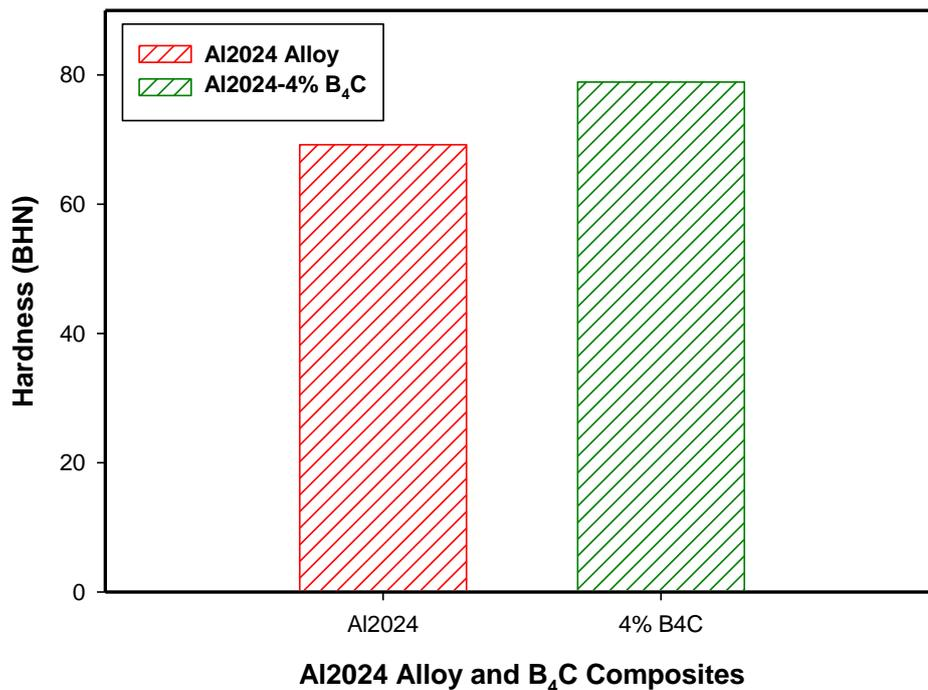
**Figure 8:** Hardness of Al2024 and 4 wt. % of micro B<sub>4</sub>C composites.
