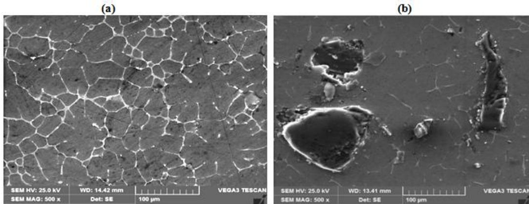
**Figure 2.** a-b Showing the scanning electron microphotographs of (a) as cast Al2024 alloy (b) with 4 wt.% of B<sub>4</sub>C.
