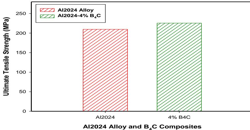
Figure 4a: Ultimate tensile strength of Al2024 and 4 wt. % of micro  $B_4C$  composites
