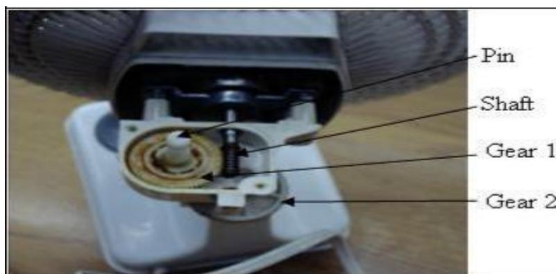
Fig. 2: Oscillating Mechanism of Standing Fan
