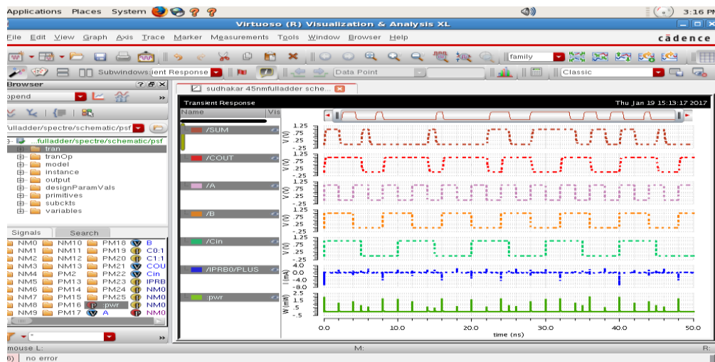
Figure 16: Output Waveform of 28T Full Adder in 45nm Technology at 50MHz frequency & 1V
