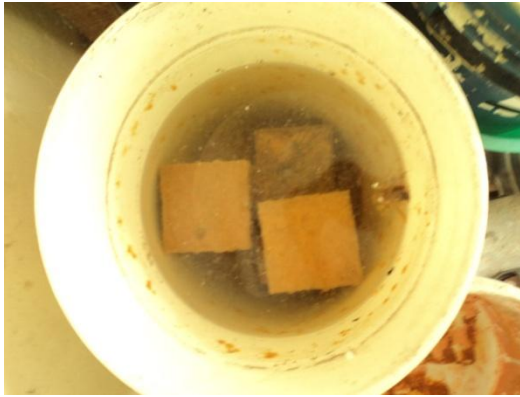
Fig.3 Cubes Exposed in Acid
