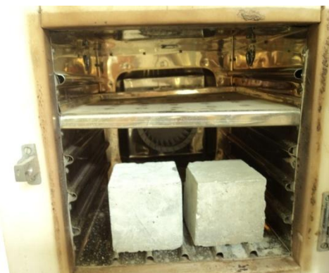
Fig.1 Placing of Cubes in Oven at 100° C
