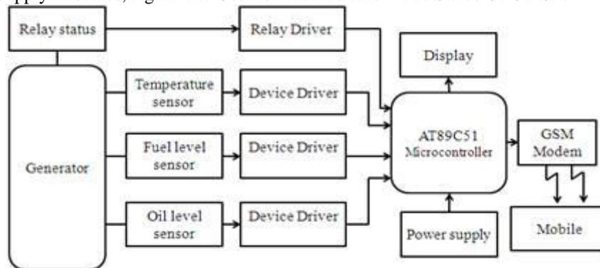
**Fig.** Block Diagram Of Proposed System
