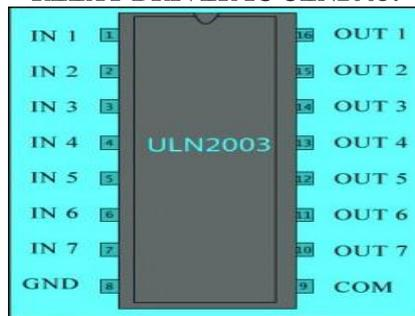
**Fig.** Pin Diagram Of Relay Driver
