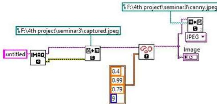
Fig 6. VI of canny edge detection
