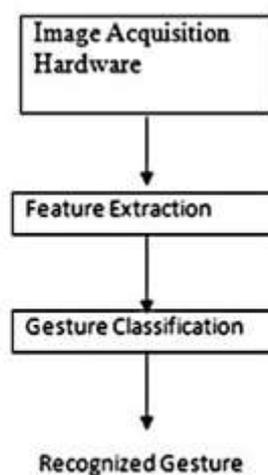
Fig.3.1 Flow diagram for gesture recognition
