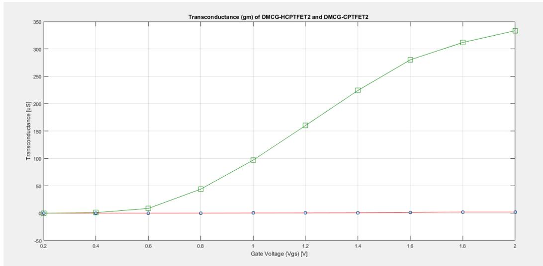
**Fig 5:** Plot for transconductance of DMCG-CPTFET2 and DMCG-HCPTFET2
