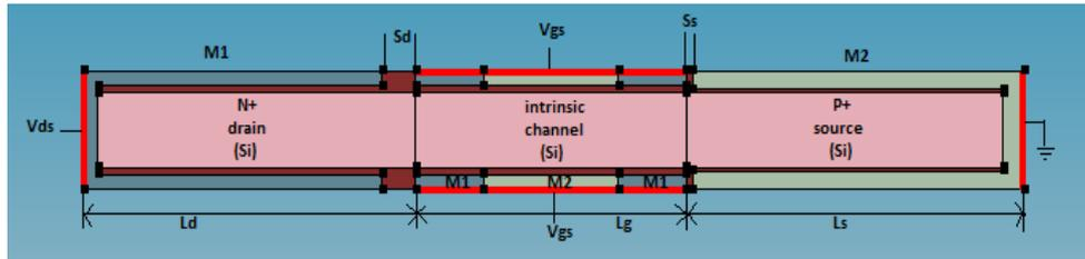
**TCAD Simulation Structure of DMCG-CPTFET2**
