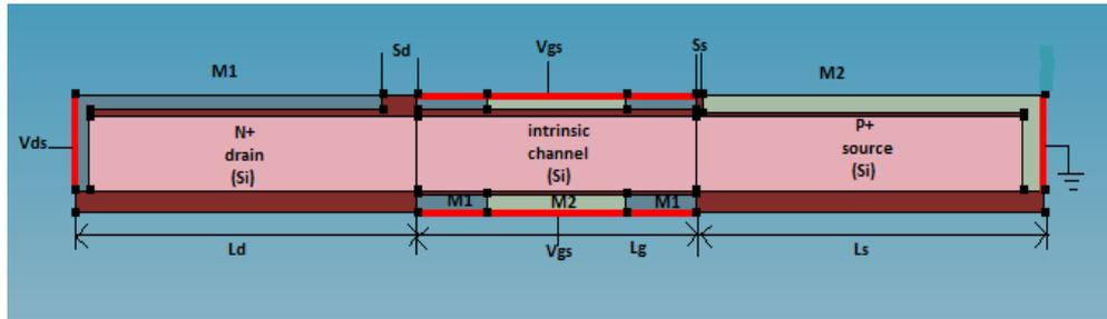
**TCAD Simulation Structure of DMCG-CPTFET1**
