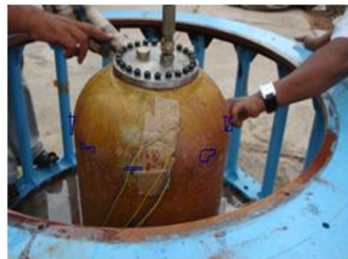
Fig.5: Test Article Along With Lvdt Position
