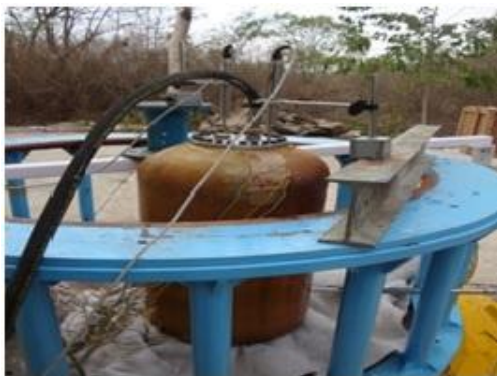
Fig. 4: Test Article Along With Strain Gauges
