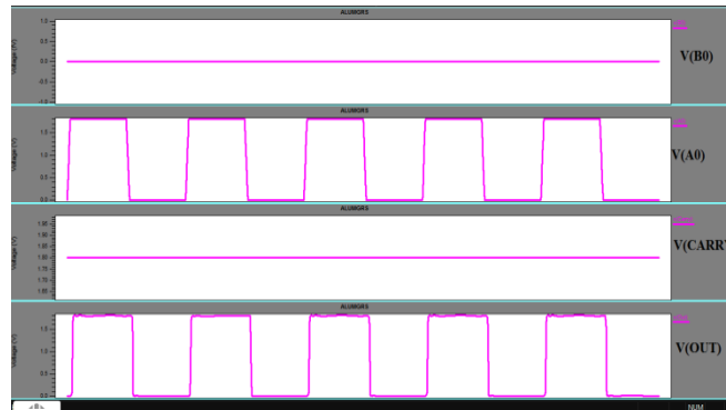
Figure (11) SUBTRACTION function of 1-bit ALU using MOD-GDI
