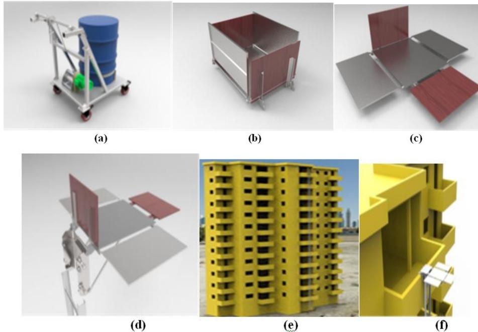
Figure3. Modeling by SOLID WORK16 (a) Rendering of balcony crane (b) rendering of material holder car closed (c) rendering of material holder open (d) Rendering of material holder guide and support assembly (e) balcony crane fully assembled isometric view (f) balcony crane with condominium building
