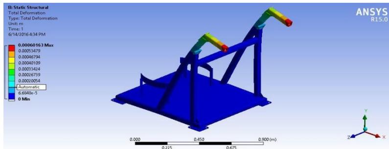
Figure 5. Frame total deformation analysis by ANSYS 15.0
