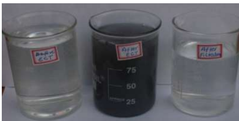
Fig. 4 Groundwater sample before ECC, after ECC and after passing through carbon filter column
