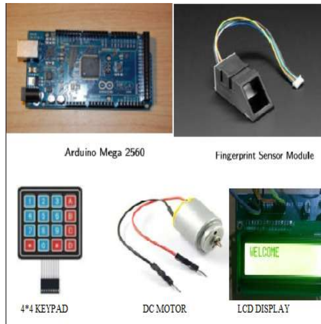
Figure 3: The Hardware Components
