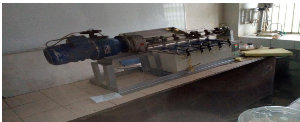
Figure 1: A locally-fabricated fermentor used for the liquefaction.
