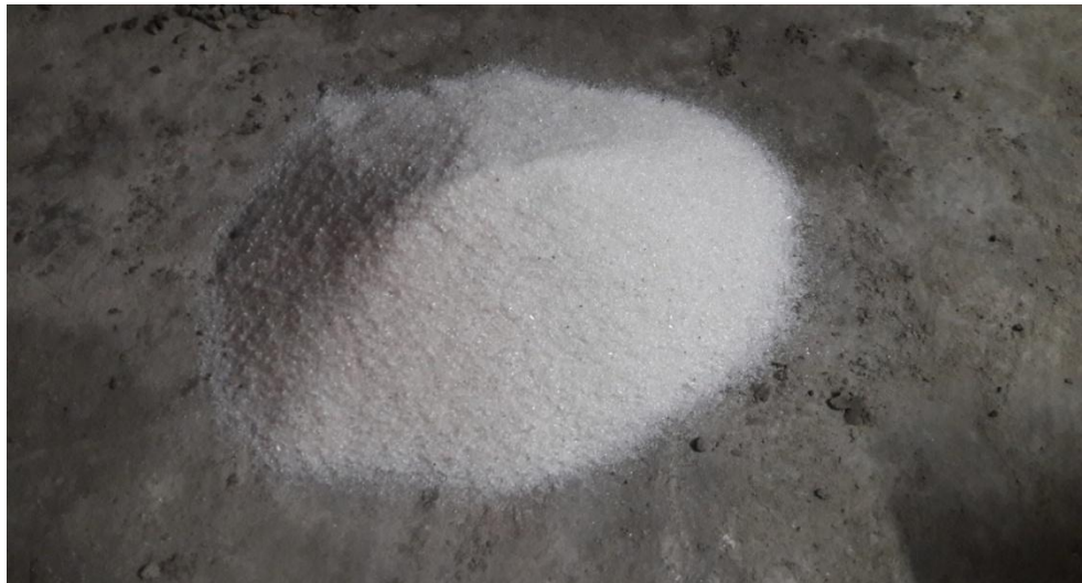
Fig: 2.1 Recycled Waste Glass as Fine Aggregate (RWGFA)
