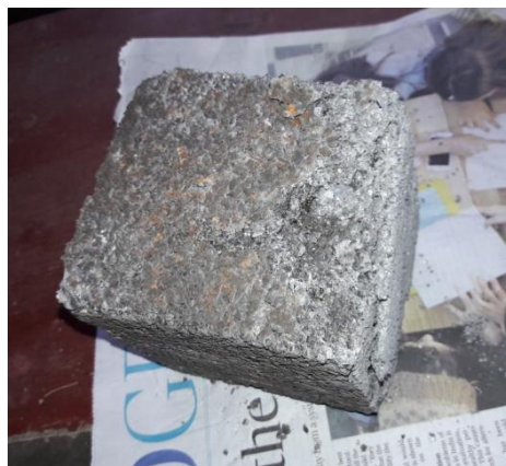
Fig: 4.1 Crack Patterns of Cubes after Testing
