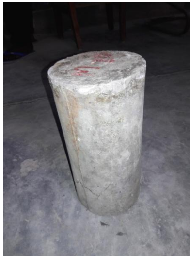
Fig: 4.4 Crack Pattern of Cylinder after Testing
