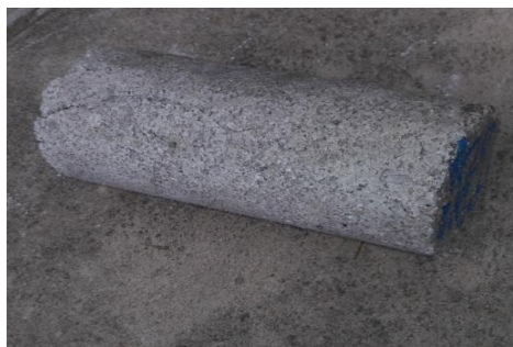
Fig: 4.2 Crack Pattern of Cylinder after Testing
