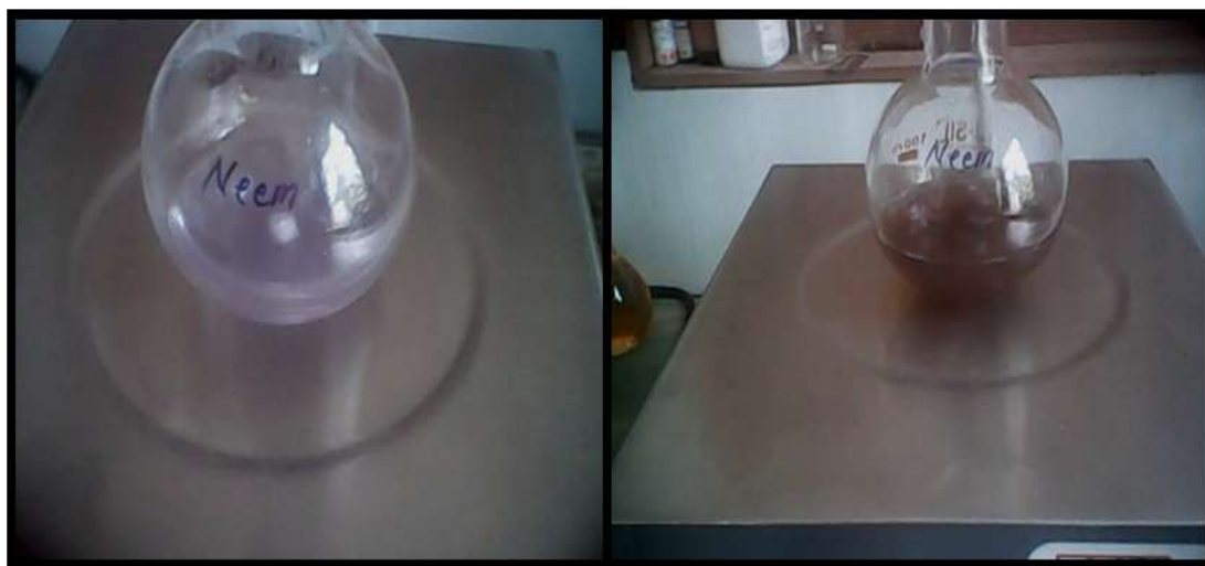
Figure 1: Solution of silver nitrate 1mmol L -1 before (left) and after (right) addition of Azadirachta indica leaf extract solution
