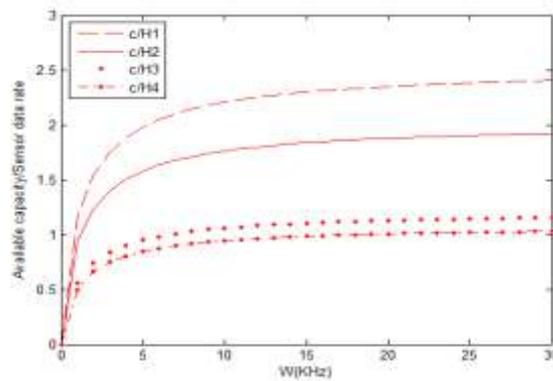
**Fig.2.** Ratio of available capacity for relays to the data collected from 3 sensors at time  $j=1$  with full operating power
