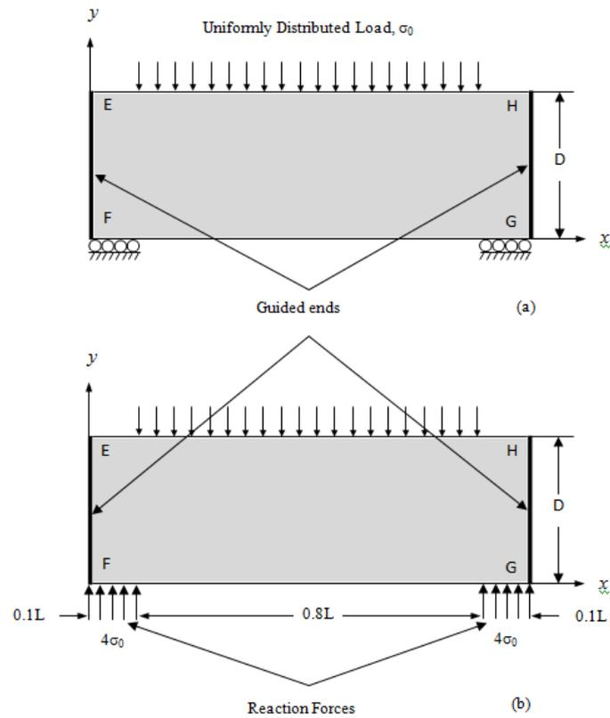
Fig. 1 (a) Physical model and (b) Analytical model of a stiffened simply-supported beam of isotropic material
