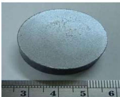
Figure 1. Forged billet of the Al-4wt.%Cu/15 vol.% Silica.
