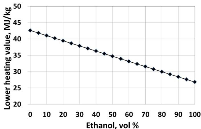
**Figure 3.** Lower heating value versus ethanol volume %.
