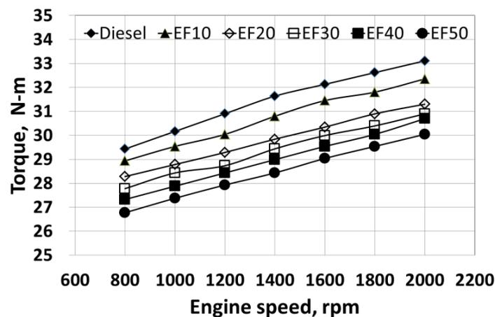
Figure 4. Torque versus engine speed for various fuels.
