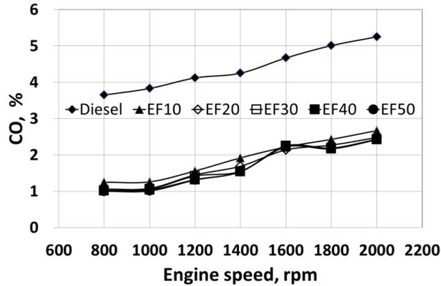
Figure 10. Carbon monoxide versus engine speed for various fuels.
