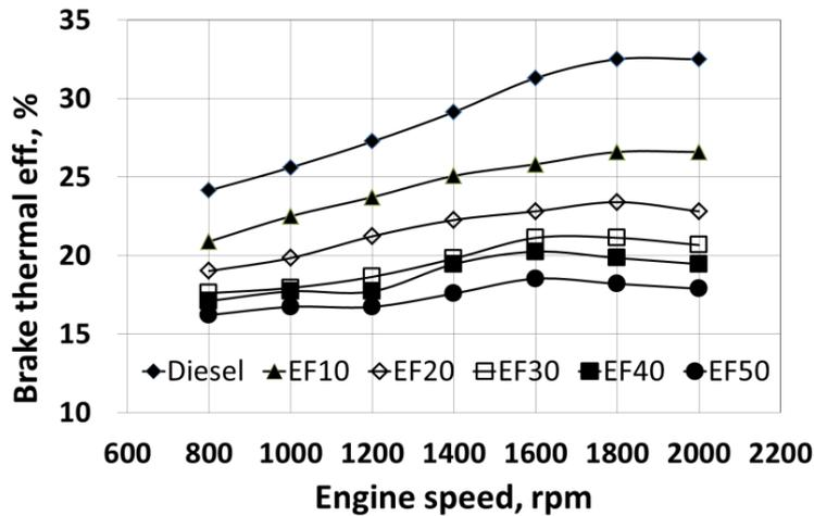
Figure 8. Brake thermal efficiency versus engine speed for various fuels.
