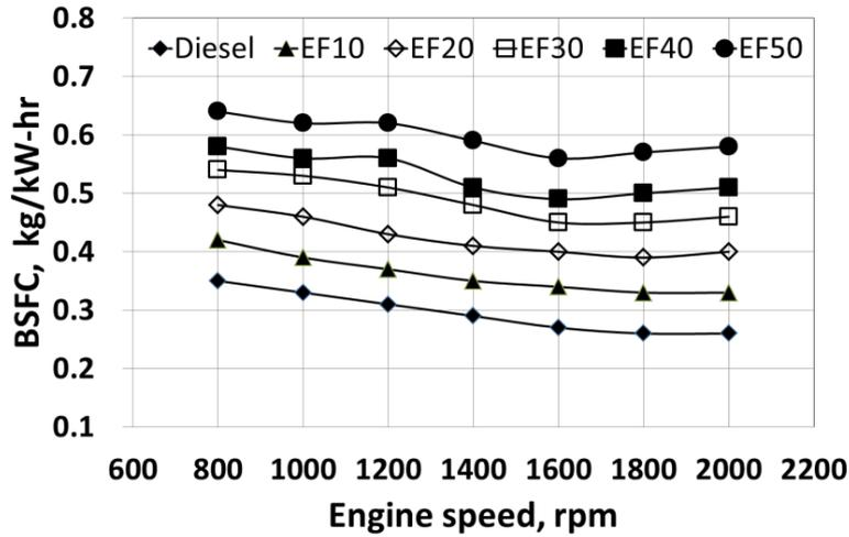
Figure 7. Brake specific fuel consumption versus engine speed for various fuels.
