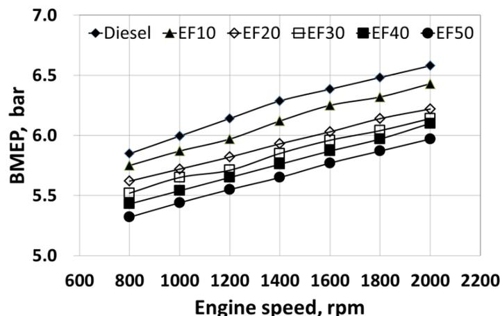
Figure 5. Brake mean effective pressure versus engine speed for various fuels.
