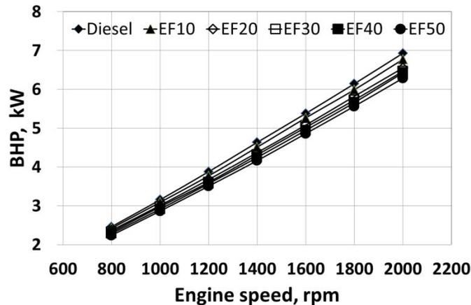
Figure 6. Brake horse power versus engine speed for various fuels.
