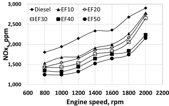
Figure 12. Nitrogen oxide versus engine speed for various fuels.
