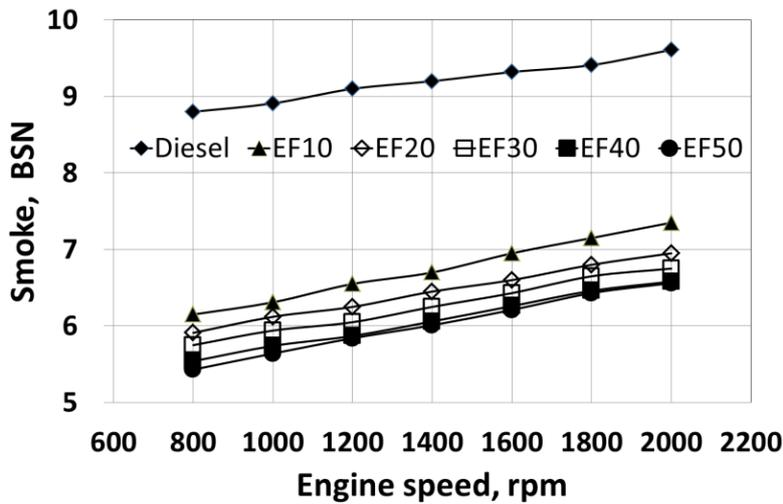
Figure 9. Smoke versus engine speed for various fuels.
