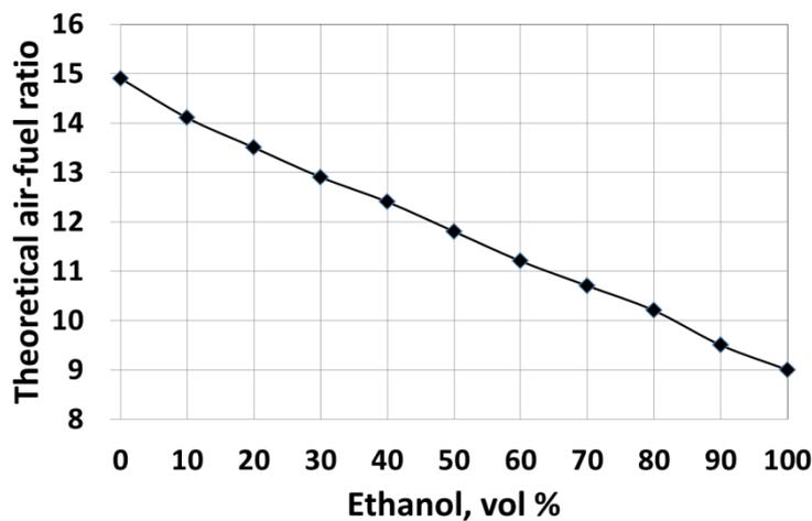
**Figure 2.** Theoretical air-fuel ratio versus ethanol volume %.
