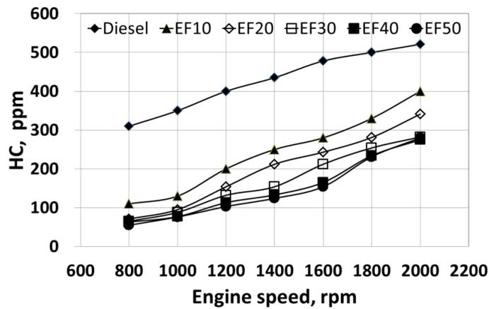
Figure 11. Hydrocarbon versus engine speed for various fuels.
