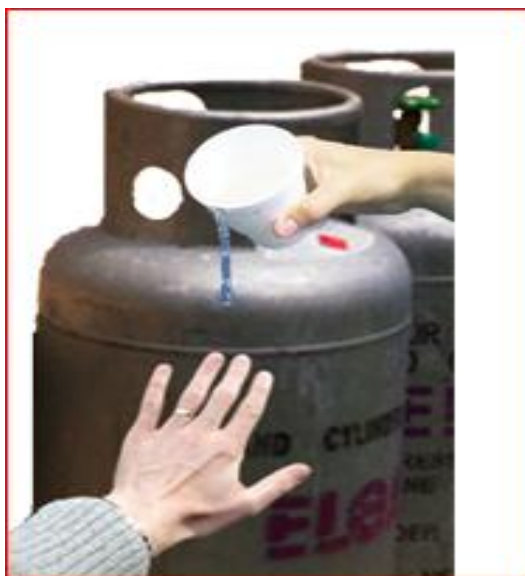
Figure 1: Checking the level of LP gas by the hand
