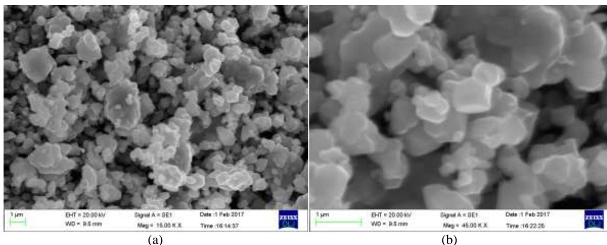
**Figure 2:** SEM images of Nickel Ferrite at (a) 15K magnification and (b) 45K magnification
