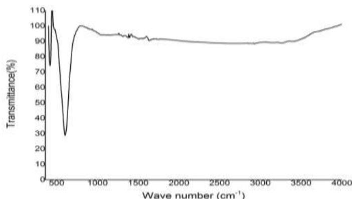
Figure 4: FTIR spectra of nickel ferrite nanoparticles.
