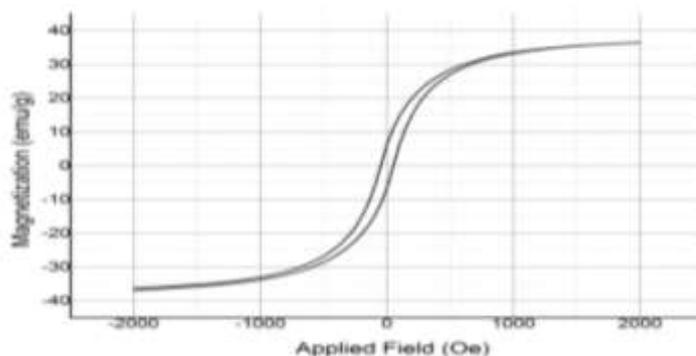
Figure 5: Magnetic hysteresis curve for nickel ferrite nanoparticles measured at room temperature.
