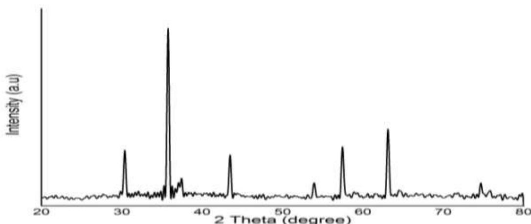
**Figure 1:** X-ray diffraction spectra of Nickel Ferrite nanoparticle.
