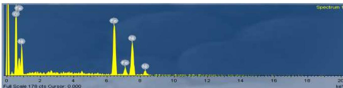
Figure 3: Energy dispersive spectroscopy (EDS) pattern of nickel ferrite nanoparticles.
