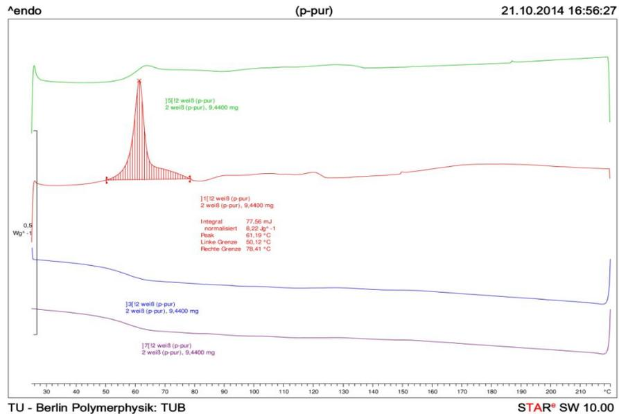
Figure 3: DSC result for thermosetting polyester/polyurethane (p-pur) powder coating residue
