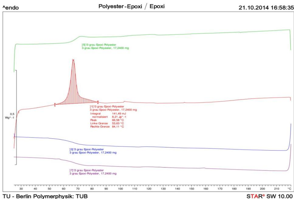
Figure 2: DSC result for thermosetting structured mixed (polyester/epoxy and epoxy) powder coating residue
