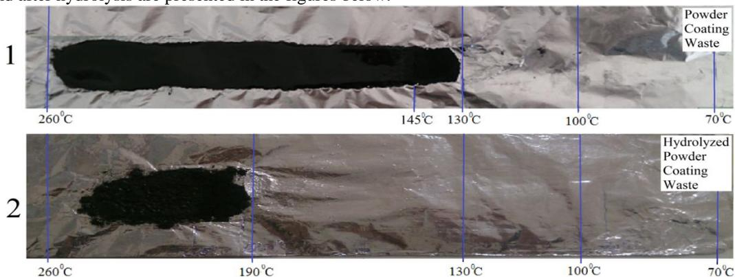
Figure 6: Hot bench results for powder coating residue consisted of polyester/epoxy and epoxy systems (1) before and (2) after hydrolysis.
