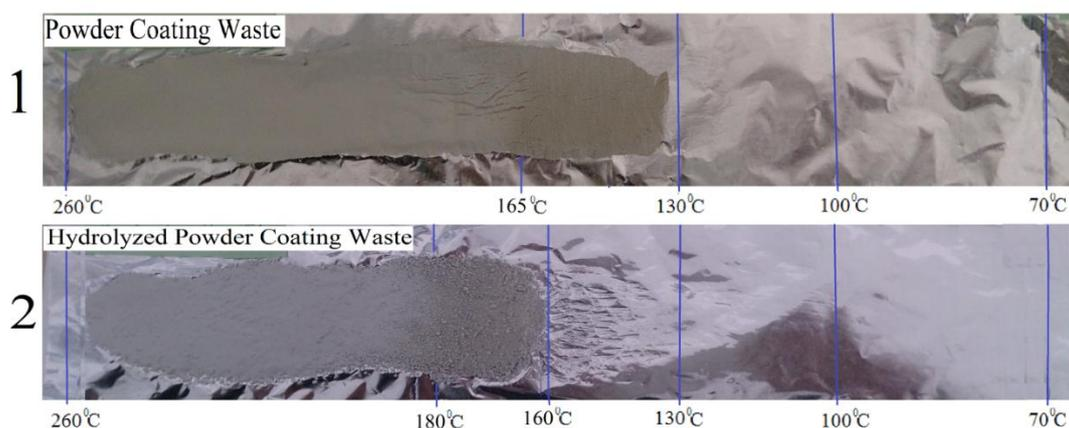
Figure 7: Hot bench results for polyester/polyurethane (p-pur) powder coating residue (1) before and (2) after hydrolysis
