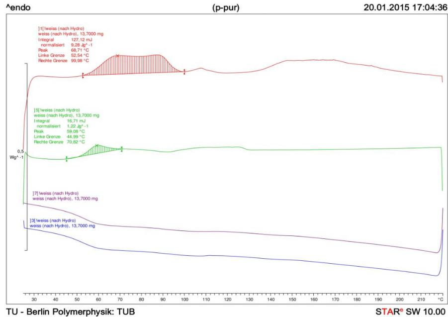
Figure 5: DSC result for hydrolyzed polyester/polyurethane (p-pur) powder coating residue
