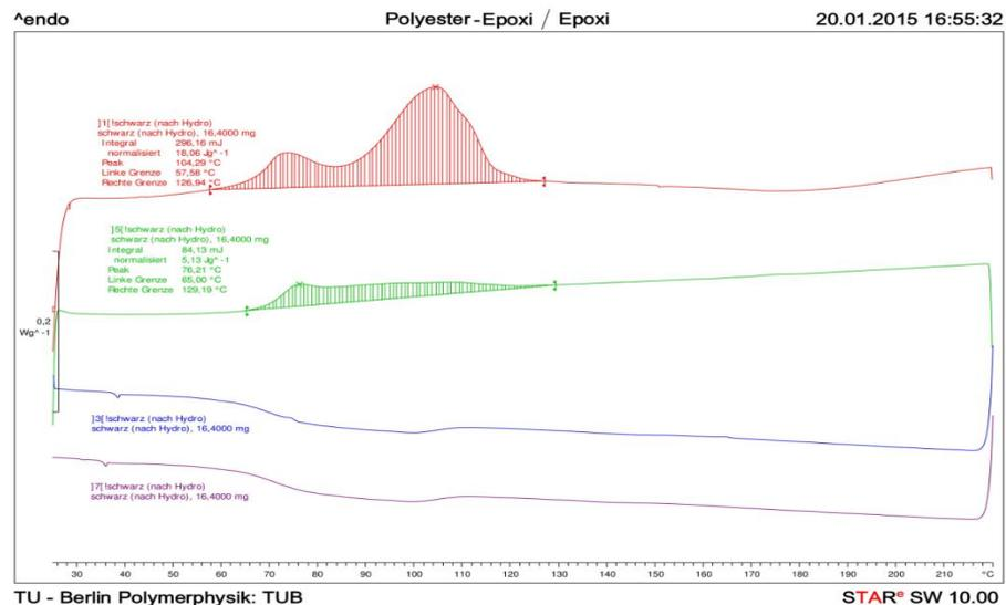
Figure 4: DSC result for hydrolyzed mixed (polyester/epoxy and epoxy) powder coating residue
