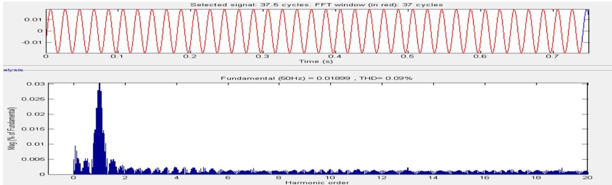
Fig 7(c).input signal and its THD analysis for capacitor supported DVR connected system
