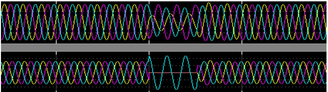
fig. 4(c) voltage swells observed at PCC voltage and load voltage
