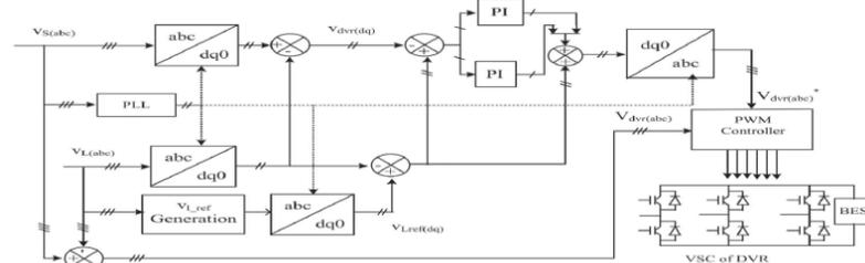
Fig.2. (b) control block of the DVR which uses SRF method of control for BESS
