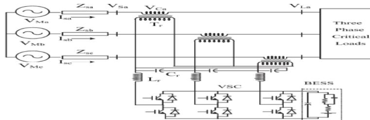
Fig.2 (a) Schematic diagram of a DVR connected system with BESS.
