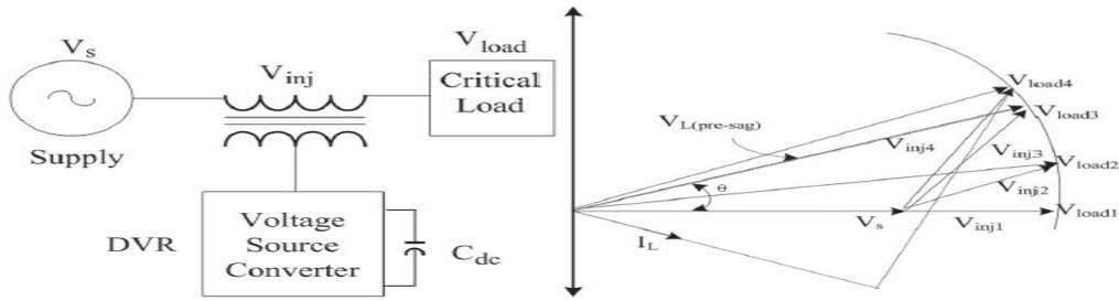
Fig. 1(a): schematic representation of DVR connected system. (b) Phasor diagram of different voltage injection schemes of DVR.
