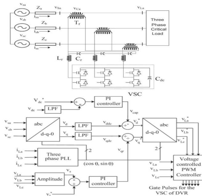
Fig.3. (a) Schematic diagram of a capacitor supported DVR connected system. (b) Control block of the DVR which uses SRF method of control for capacitor connected DVR
