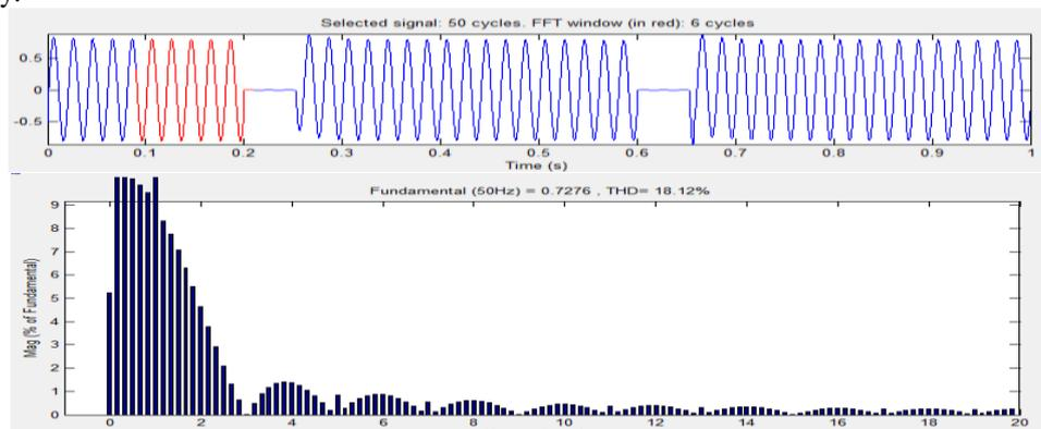
Fig 7(a).input signal and its THD analysis for DVR connected system with BESS without control
