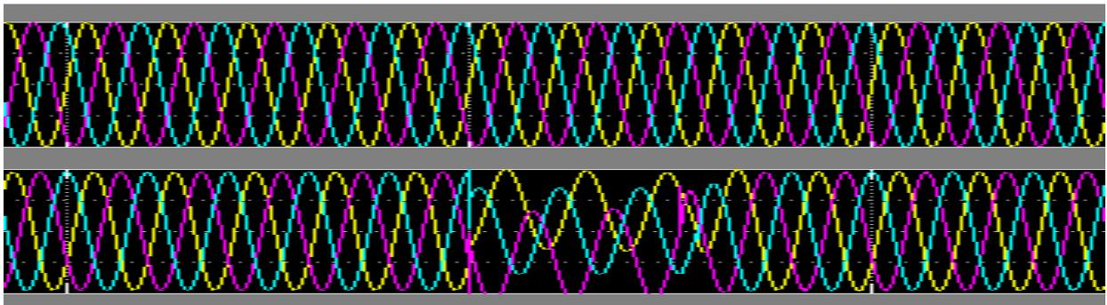
fig. 5(a) voltage sags compensated at PCC voltage and load voltage
