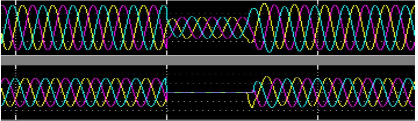
fig. 4(b) voltage sags observed at PCC voltage and load voltage
