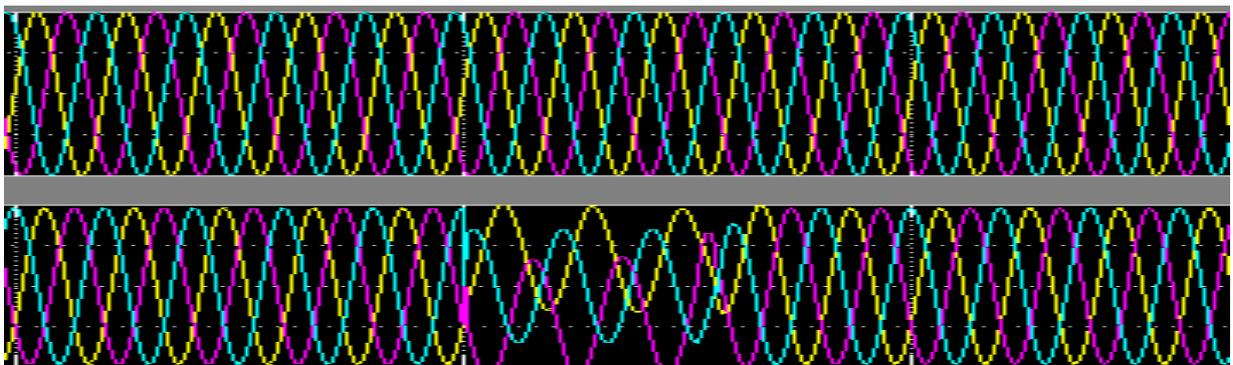
fig. 5(b) voltage swells compensated at PCC voltage and load voltage
