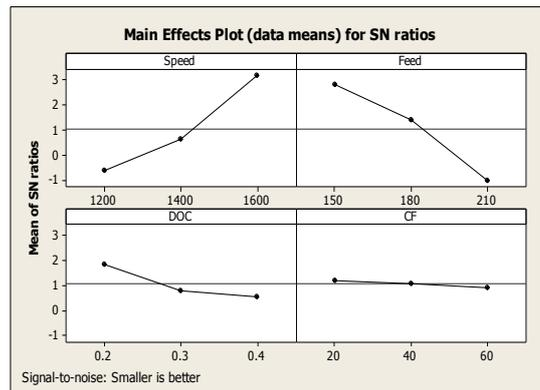
**Fig 1. Effects of process parameters**
