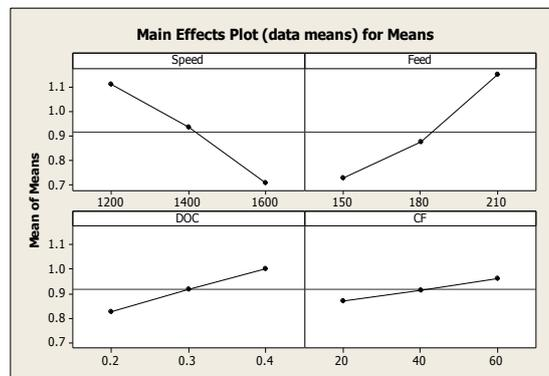
**Fig2.Effects of process parameters on means on S/N Ratios**
