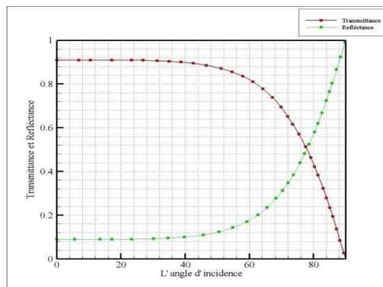
Fig.4 Transmittance and reflectance evolution as a function of angle of incidence ( $i$ ).
