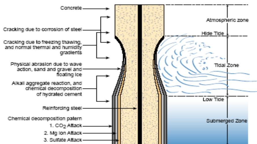
**Figure 1: Concrete Cylinder Exposed to Seawater**
