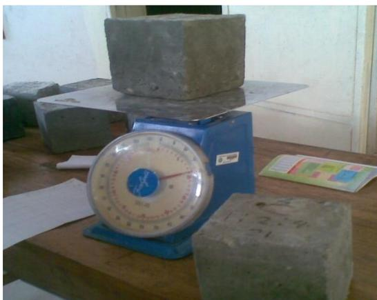
Fig 4: Weighing of Cube
