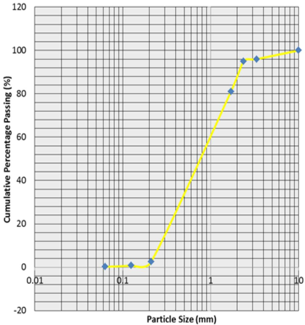
**Figure 6: Particle Size Distribution of Fine Aggregate**
