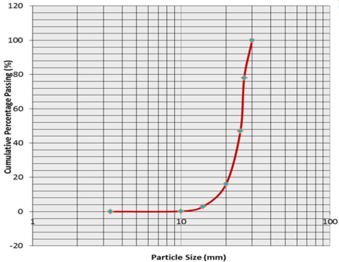
**Figure 7: Particle Size Distribution of Coarse Aggregate**
