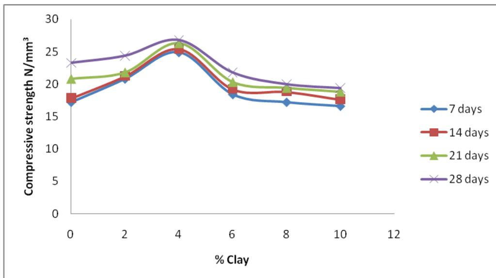
Fig.1: Relation between compressive strength of concrete and percentage clay
