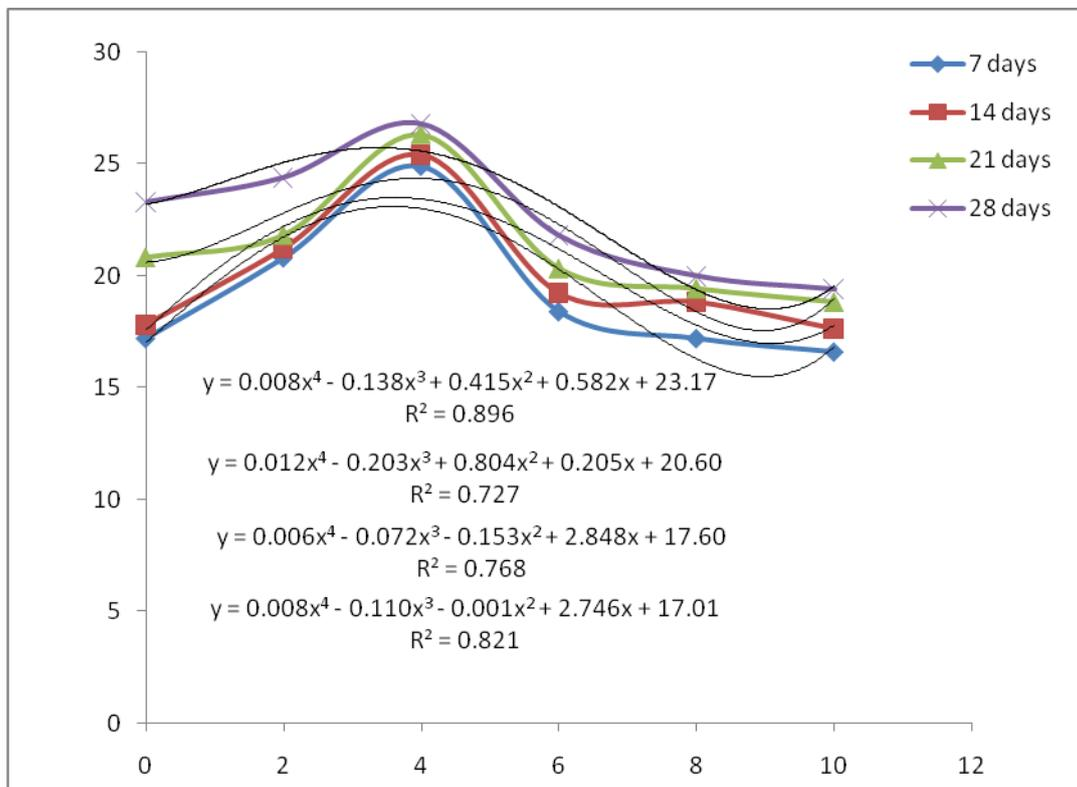
**Fig.3: Trend of compressive strength with increase percentage clay**
