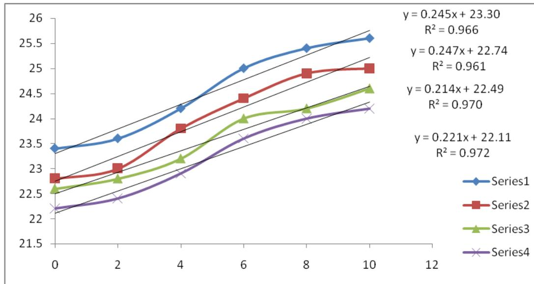
**Fig. 4: Trend of density with increase percentage clay and drying days**
