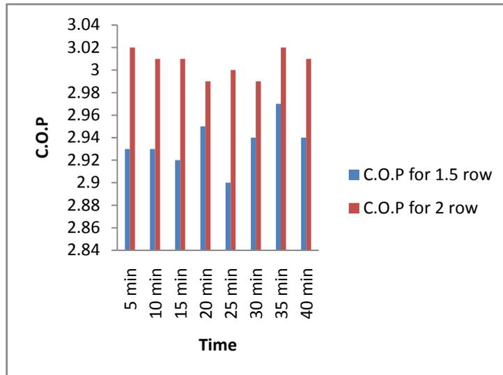
Fig-14: Graphical representation of C.O.P with 1.5 Row and 2.0 Row Fin Tube Condenser heat Exchanger.
