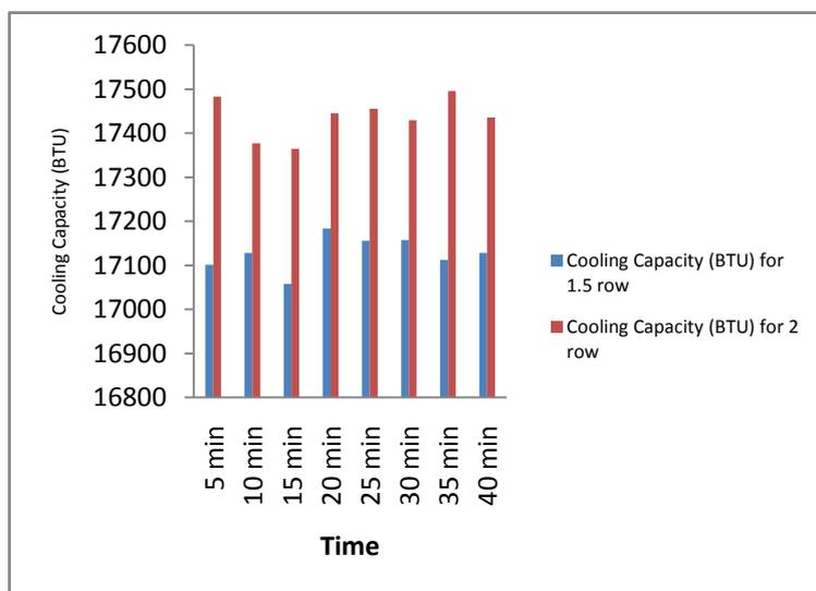
Fig-13: Graphical presentation of Cooling Capacity for 1.5 row and 2 row condenser with respect to time.
