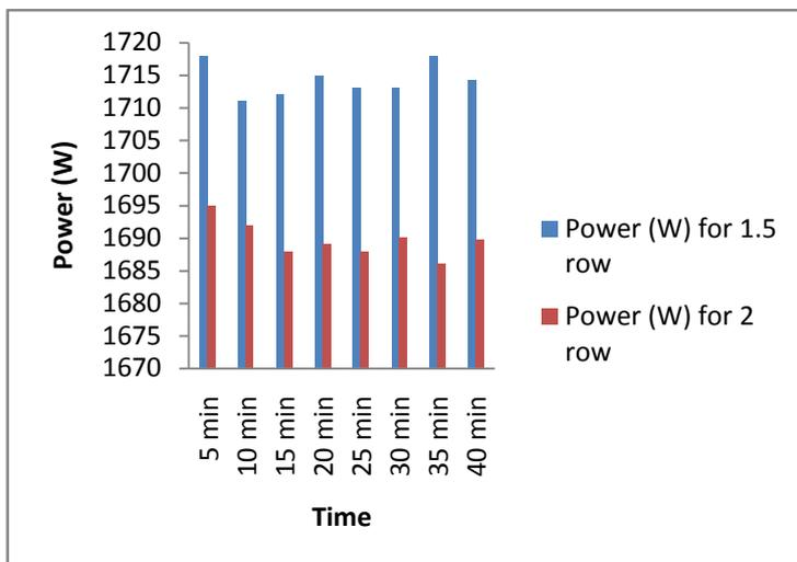
Fig-12 : Graphical presentation of the power for 1.5 row and 2 row condenser
