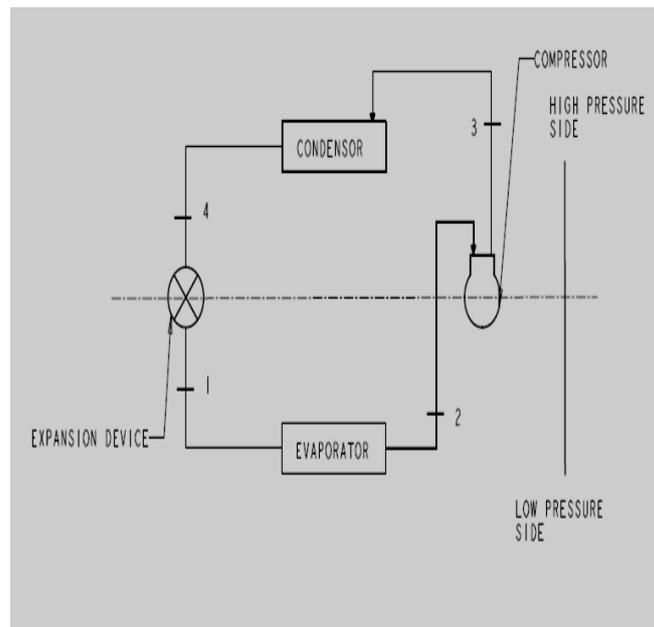
Fig- 2: Schematic representation of the vapour compression refrigeration cycle[2]
