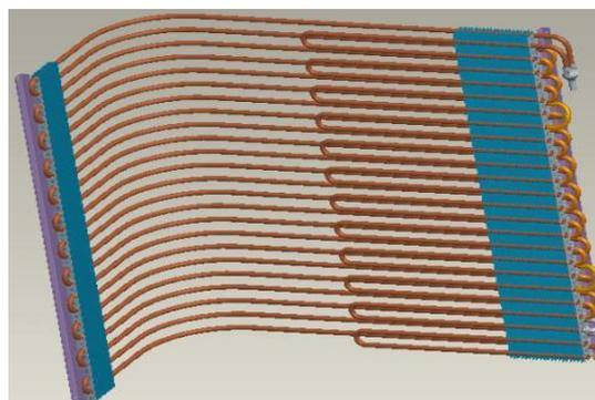
Fig- 4: Typical Plate Finned-Tube Heat Exchanger
