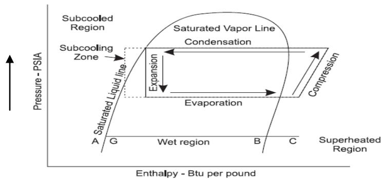
Fig-3: Schematic representation of the refrigeration cycle including pressure change.
