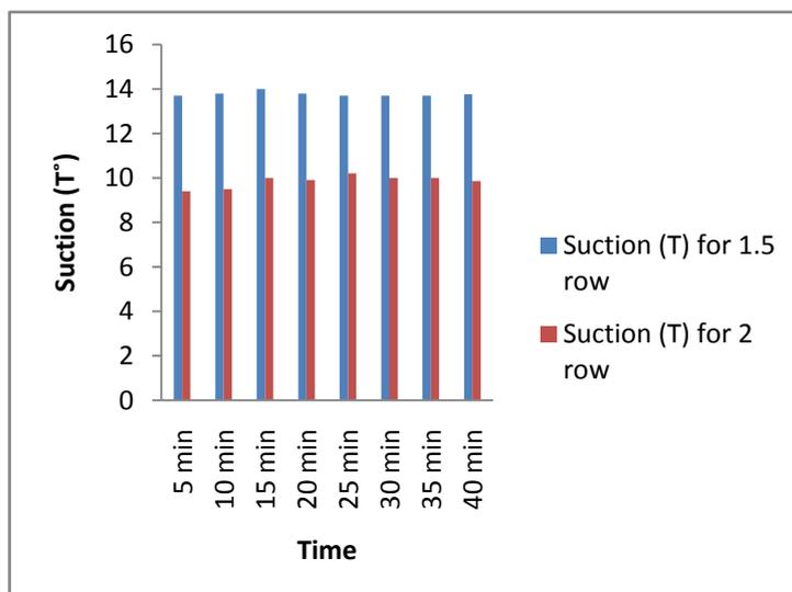
Fig-15: Graphical representation of Suction temp. of 1.5 Row and 2.0 Row Fin Tube Condenser heat Exchanger.
