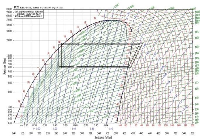
Fig-10: P-H diagram of FIN tube heat condenser with 1.5 row and 2.0 row coil on the cooling of 1.5TR split air conditioner.
