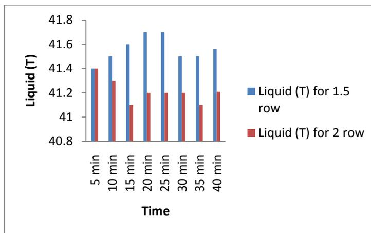
Fig-17: Graphical representation of liquid with 1.5 Row and 2.0 Row Fin Tube Condenser heat exchanger.
