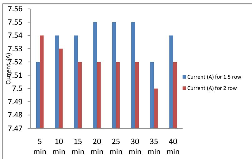
Fig-11: Graphical presentation of the current for 1.5 row and 2 row condenser
