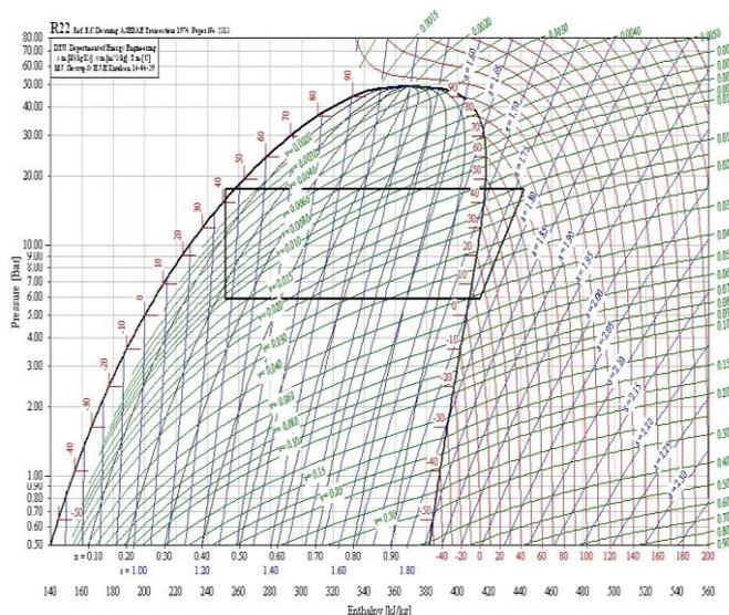
Fig-8: P-H diagram of FIN tube heat condenser with 1.5 row coil on the cooling of 1.5TR split air conditioner.
