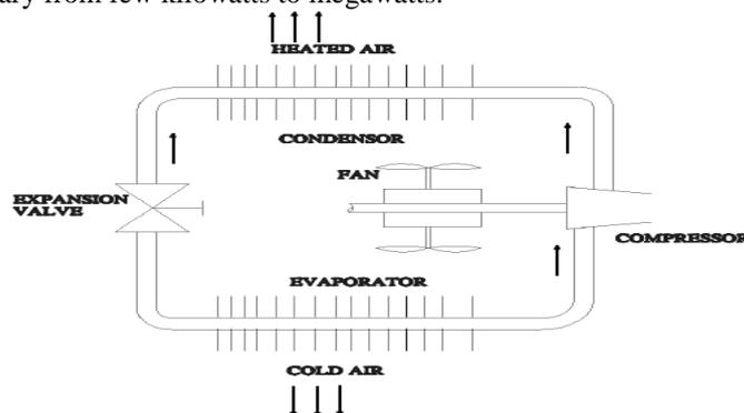
Fig-1: Schematic of a basic vapor compression refrigeration system[1]
