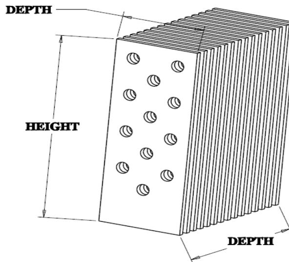
Fig-7: Layout of Heat Exchanger Geometry Parameters[23]
