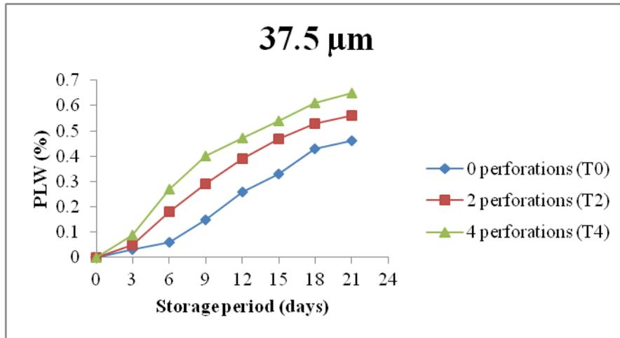
Figure 4: PLW (%) for 37.5 μm thickness LDPE film under low temperature storage conditions
