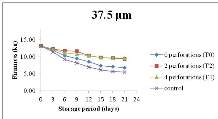
Figure 8: Firmness (kg) for 37.5 µm thickness LDPE film at low temperature storage
