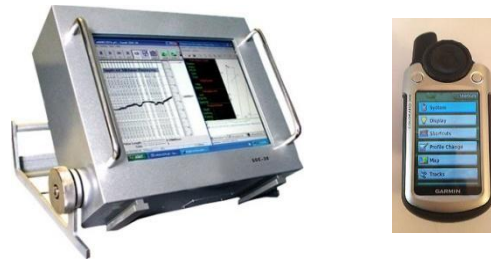
Figure 3: Echo Sounder and GPS Instrument Used
