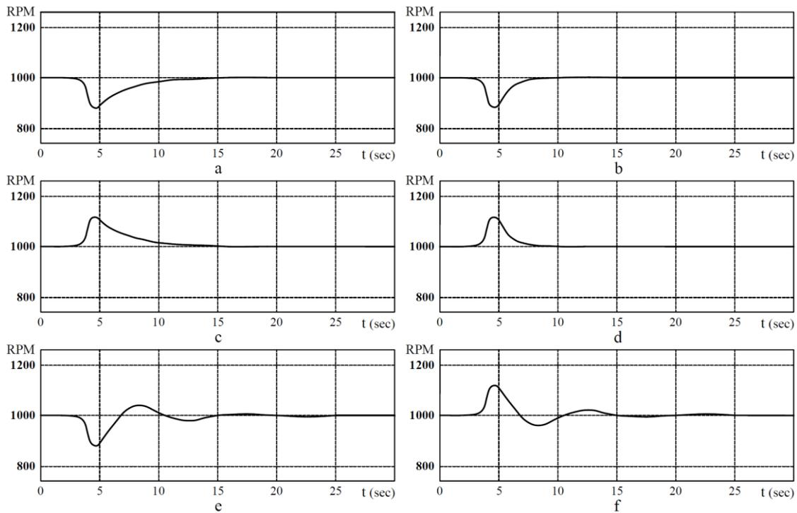
Fig. 2. Examples of transient processes in turbine RPM control during load connection/disconnection
