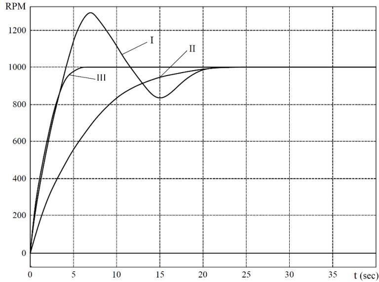
Fig.1. Examples of transient processes in turbine RPM control during the startup of HPP units
