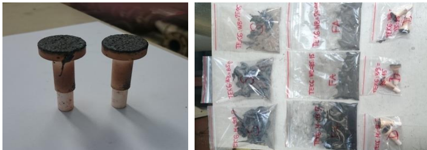
Figure 7. Samples of deposits and slag during co-firing of biomass with coal K2 - see also [21].
