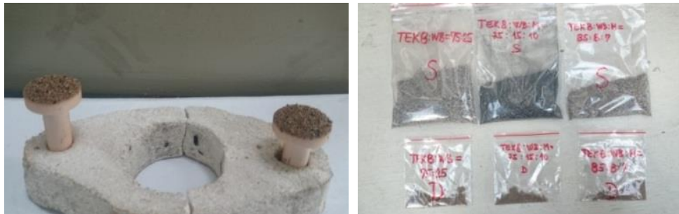
Figure 4. Samples of deposits and slag during co-firing of biomass with coal K1 - see also [21].
