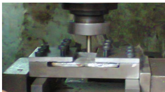
Fig 2.1 shows the fixing of work pieces on the bed of milling machine by using fixture
