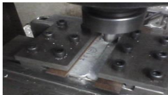
Fig 2.2 shows the fixing of tool in the spindle and the probe inserted into the work piece
