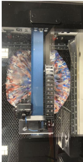
Figure 6. Recycled sheet inside laser engraver
